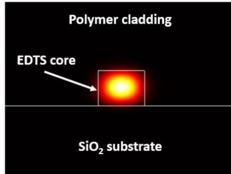
Figure 5. Channel waveguide cross-section based on a hybrid glass-polymer structure
