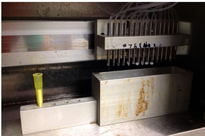
*Figure 79. Reaction chamber of the MerMade 4 synthesis machine. Visible at the top right of the image are the reagent injection nozzles that move to the left to deliver reagents to the yellow synthesis column. Visible on the ends of the nozzles is build up of crystallised activator, which prevented reliable delivery of activator during synthesis of long oligonucleotides.*
