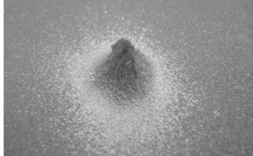
Figure 16 - Pyramid deposit formed by masked cold spray [53]
