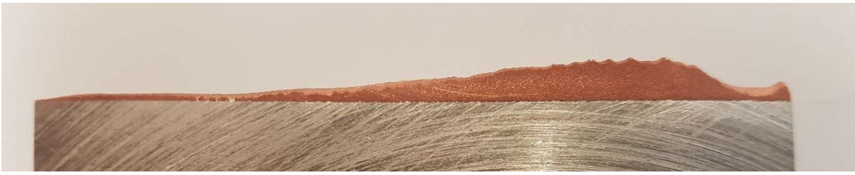
Figure 43 - Successful copper deposition against 10 mm backstop, at a steady declining traverse rate from 25 to 3.75 mm/s
