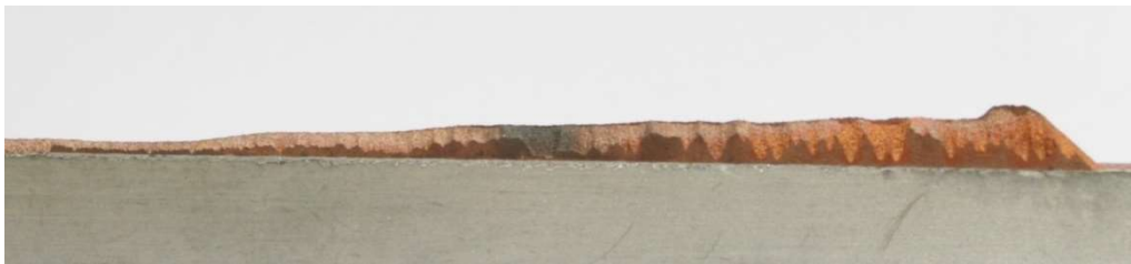
Figure 44 – Failed copper deposition adjacent to 10 mm height backstop at 25, 15, 7.5, 5 and 3.75 mm/s
