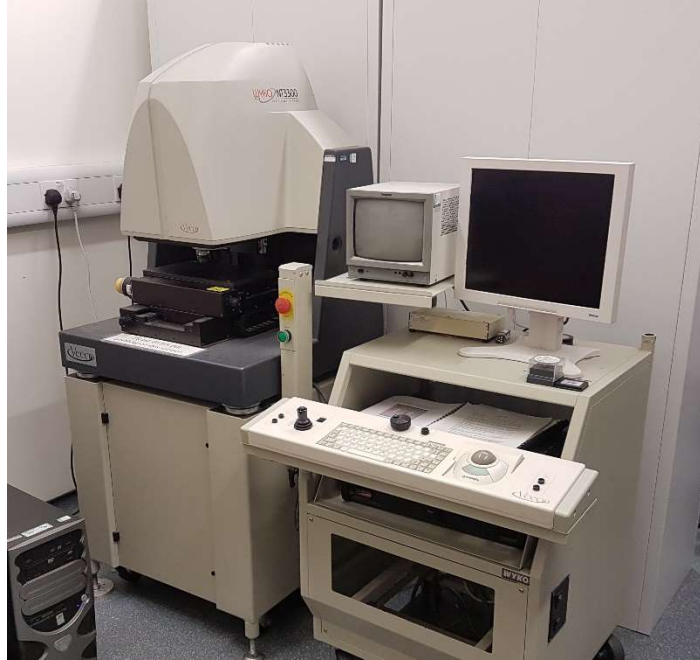
Figure 33 - Veeco Wyko NT3300 used for surface roughness measurements
