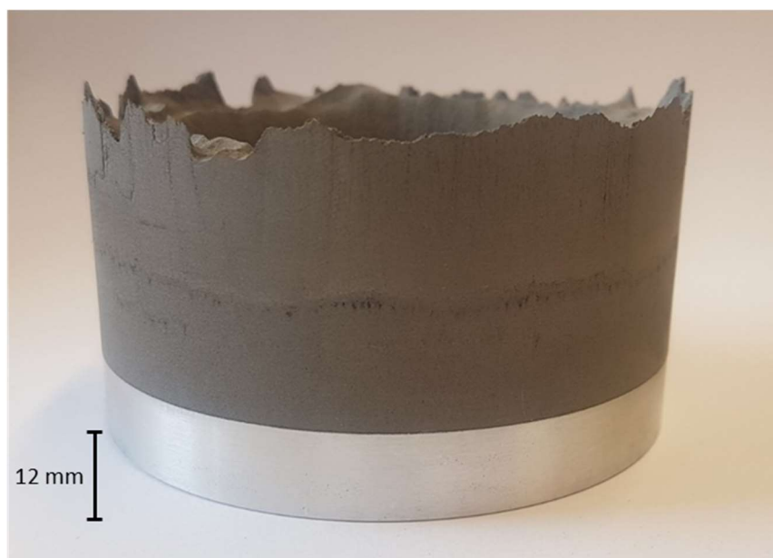
Figure 109 – Deposited titanium tube, 55 mm height, 89 mm diameter
