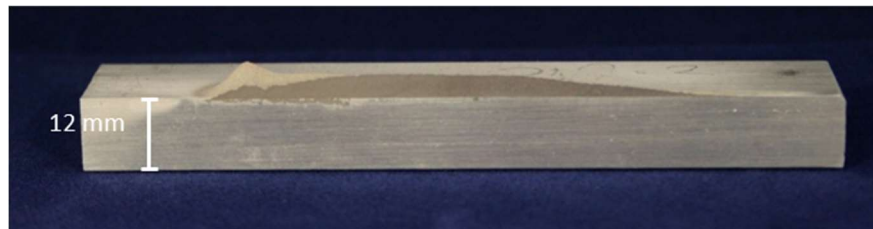
Figure 88 – Build profile of steel nozzle alignment test
