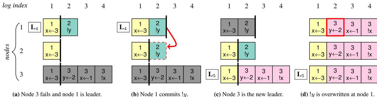
**Figure 6:** Example of Leader Completeness violation, without the extra condition on commitment. The entry !y at index 2, term 2 is committed by node 1 (the leader in term 4) but later overwritten by node 3 (the leader in term 5). Grey logs correspond to failed nodes.
