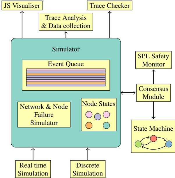
Figure 1: Overall architecture of our simulator.
