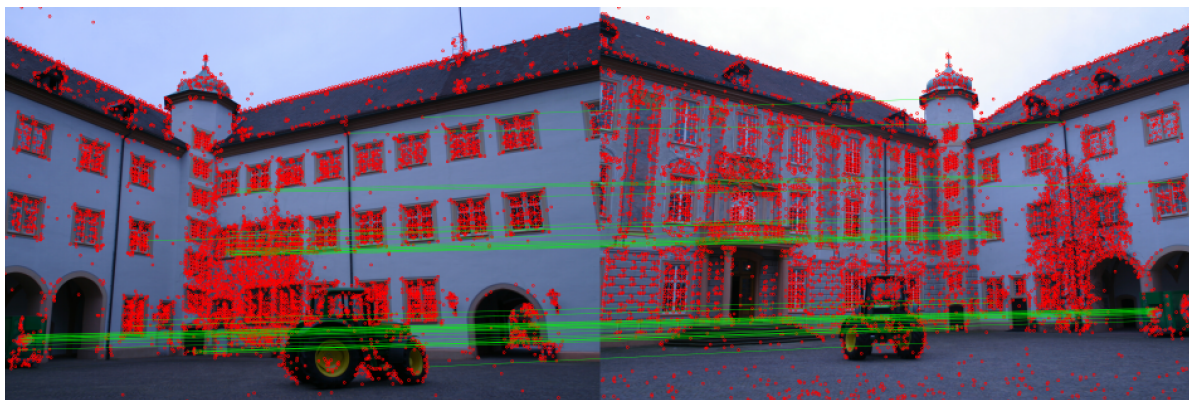
Fig. 2.6 An example of false inlier matches after 2-view geometric verification due to repetitive structures. Each red point denotes a SIFT feature. This image was drawn using COLMAP [Schönberger and Frahm, 2016].
