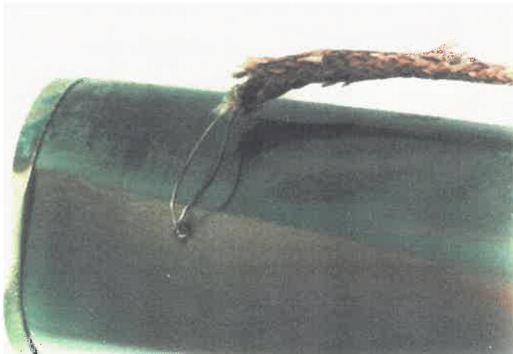
Fig. 7.6. Photograph showing the position of the thermocouple on the wear scar at an impact velocity of  $2.1 \text{ m s}^{-1}$ , the back of the specimen is at the top of the picture.
