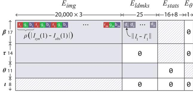
**Figure 8:** The non-zero structure of our Jacobian  $J_T$  for a  $200 \times 100$ px eye region.  $J_T$  is calculated entirely on the GPU. Dashed regions represent sparse blocks.
