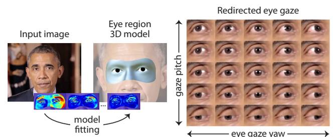
**Figure 1:** *GazeDirector* is a new 3D model based approach for gaze redirection. We first recover the shape and appearance of the eyes by fitting a 3D eye region model. We then redirect gaze by warping the eyelids and rendering new redirected eyeballs. Examples of redirected gaze can be seen on the right.
