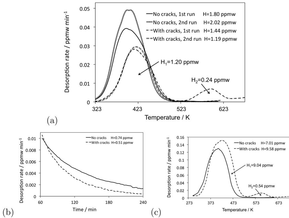
Figure 2: a) Experiment 1: Desorption during ramped heating at  $100 \text{ K h}^{-1}$  ( $100^\circ \text{C h}^{-1}$ ) after 7 h charging (recharged once), b) Experiment 2: Isothermal desorption at 363 K ( $90^\circ \text{C}$ ) for 4 h after 7 h hydrogen charging (no recharging), c) Experiment 3: Desorption during ramped heating at  $100 \text{ K h}^{-1}$  ( $100^\circ \text{C h}^{-1}$ ) after 120 h charging, (no recharging).
