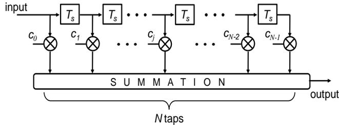
Figure 2. Schematic of a finite impulse response filter.
