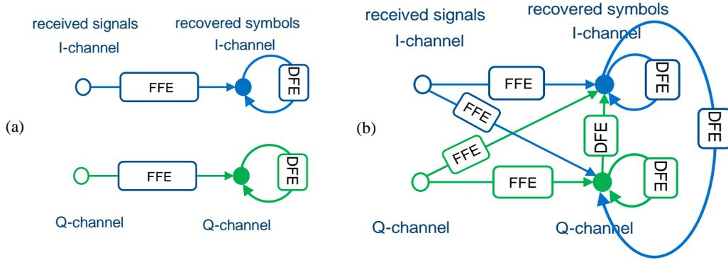
Figure 3. Schematic of the structure of (a) conventional FFE and DFE equalizer and (b) the CAP equalizer.
