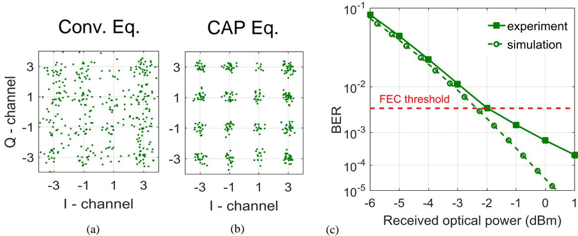
Figure 8. Noise-free constellation diagrams for 112 Gb/s CAP-16 data transmission over 100 m OM4 for the (a) conventional and (b) CAP equalizer and (c) BER curves for the CAP equalizer.
