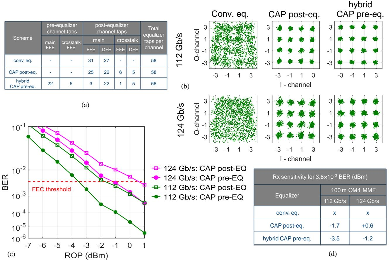
Figure 9. (a) Number of taps used for each part of the three equalizers studied for the data transmission of 112 and 124 Gb/s CAP-16 over 100 m OM4 (b) respective noise-free constellation diagrams, (c) estimated BER curves for the operating links (CAP post-eq. and hybrid CAP pre-eq.) and (d) receiver sensitivity for the HD FEC threshold.
