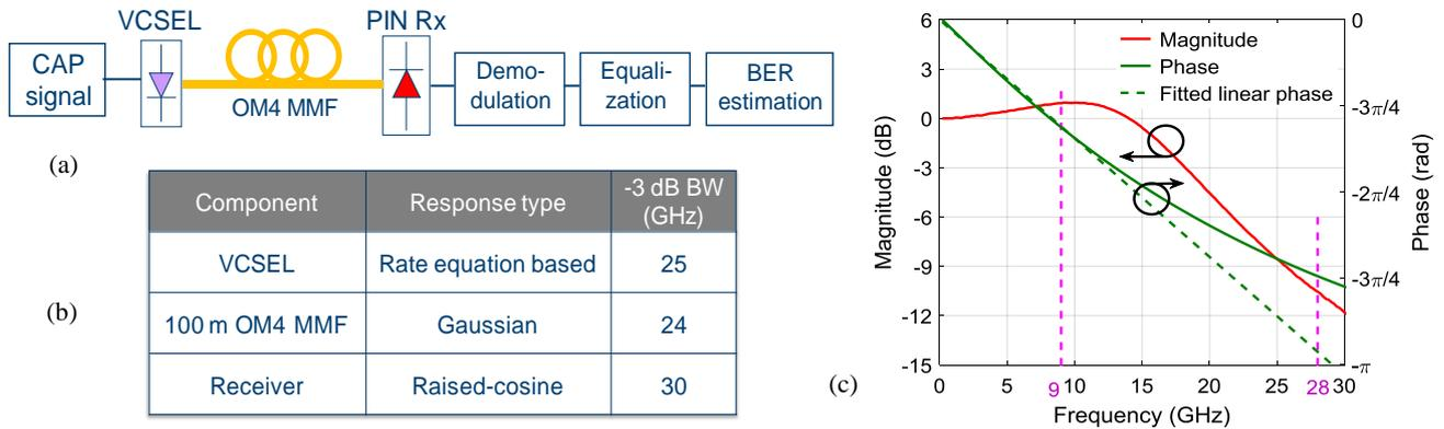
Figure 4. (a) Illustration of link model used in the simulation studies, (b) main component parameters and (c) total link amplitude and phase response.
