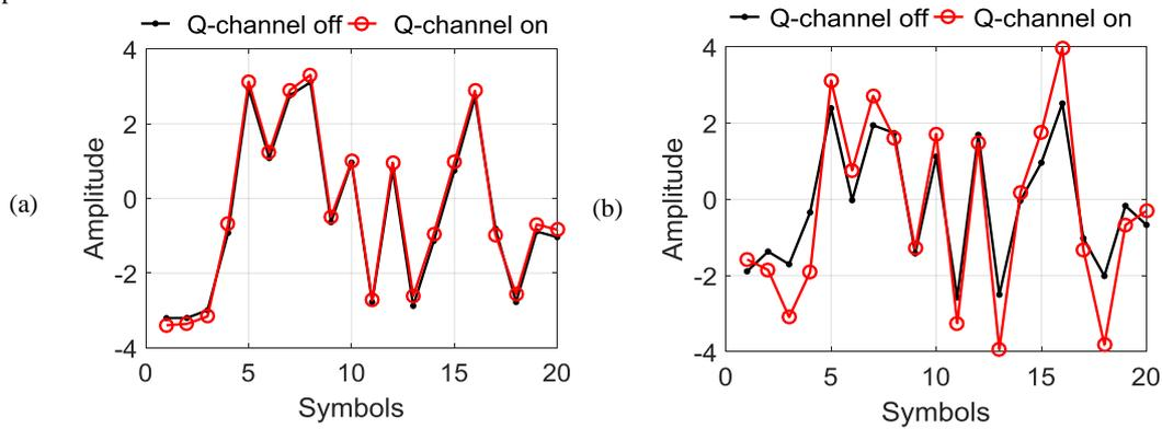
Figure 5. Received symbol amplitude for the I-channel for CAP-16 data transmission over 100 m OM4 when the Q-channel is and is not transmitting data at (a) 9 GBaud (36 Gb/s) and (b) 28 GBaud (112 Gb/s).
