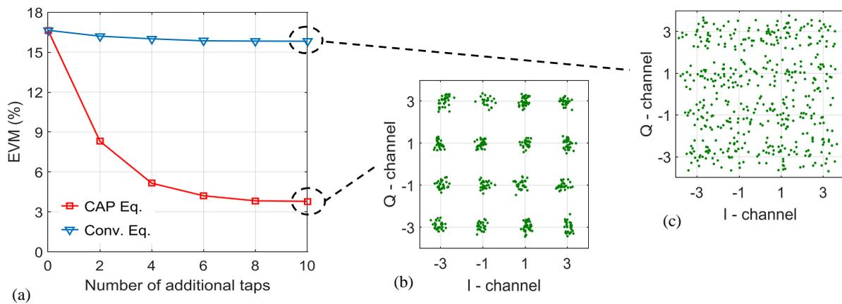
Figure 6. (a) EVM of the received signal for 112 Gb/s CAP-16 100 m OM4 data transmission as a function of the number of additional taps used on each channel for the two types of equalizers and (b-c) noise-free constellation diagrams of the recovered symbols for the longest equalizer considered (50 taps in total on each channel): (b) CAP and (c) conventional equalizer.
