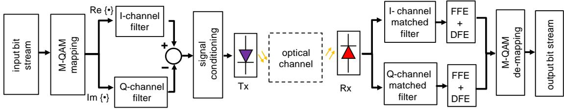
Figure 1. Diagram of a typical CAP-based transmission scheme.
