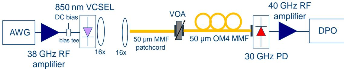
Figure 7. Experimental setup used in data transmission studies.
