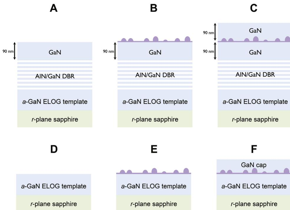
**Fig. 1.** Schematic diagram of the structures of sample A – F. Sample A – AlN/GaN DBR and a 90 nm GaN; Sample B – uncapped InGaN QD layer on DBR +90 nm GaN; Sample C – InGaN QDs at the centre of 180 nm GaN layer on top of DBR; Sample D – *a*-plane ELOG template on *r*-plane sapphire; Sample E – uncapped InGaN QD directly grown on top of ELOG; Sample F – capped InGaN QDs on ELOG template.
