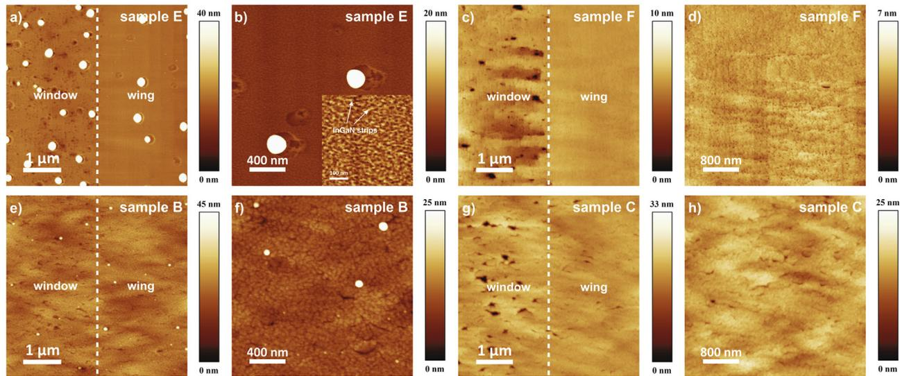
**Fig. 3.** AFM images of a) sample E and e) sample B – uncapped InGaN QD layer, and c) sample F and g) sample C – capped InGaN QDs with a GaN cap grown on top of GaN ELOG pseudo-substrates on top of an AlN/GaN DBR, respectively. b), d), f), and h) are zoomed in images taken from the low-defect density wing regions of a), c), e) and g) respectively.
