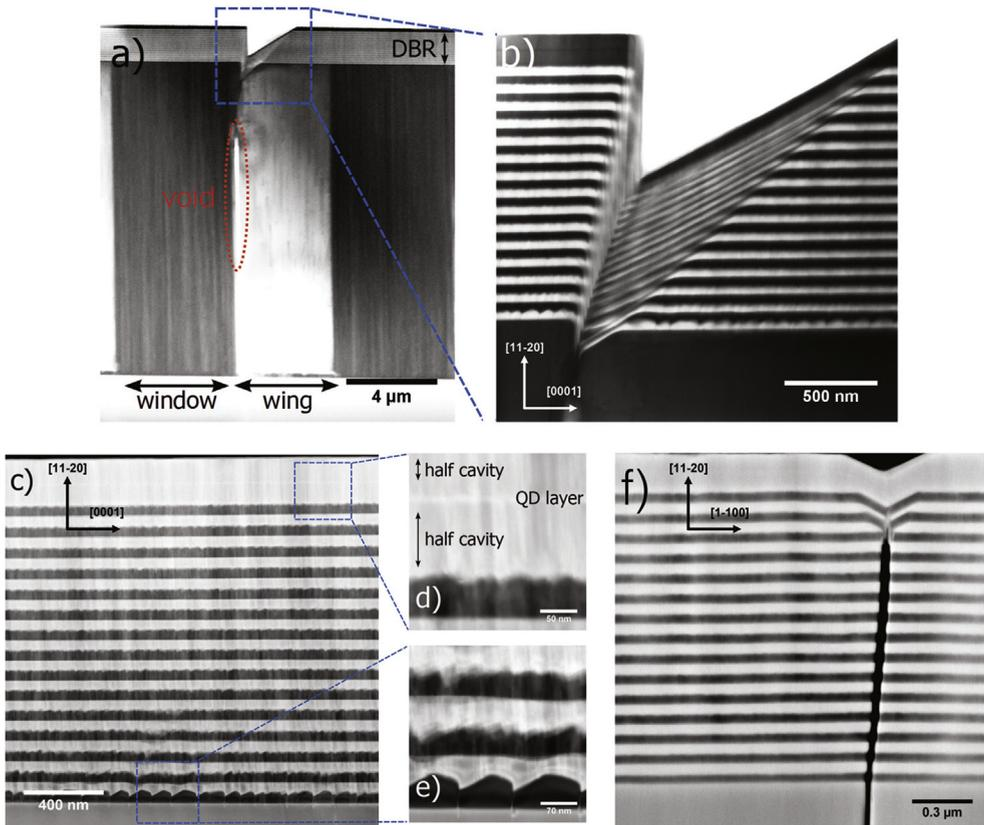
**Fig. 5.** Cross-sectional STEM images of sample C - the capped QD sample grown on top of a 15-period AlN/GaN DBR. a,b) BF-STEM images; c,d,e) HAADF images viewed along [1–100], whilst f) is viewed along [0001].
