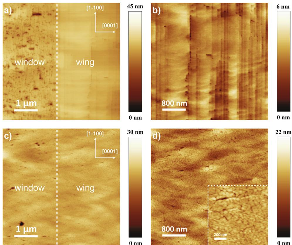
**Fig. 2.** AFM images of a) Sample D – *a*-plane GaN ELOG template, c) Sample A – a 15-period AlN/GaN DBR on *a*-plane GaN ELOG with a 90 nm GaN layer. Zoomed in images taken from the low-defect density wing regions b) and d), Inset: 1 × 1 μm<sup>2</sup> scan from the wing.
