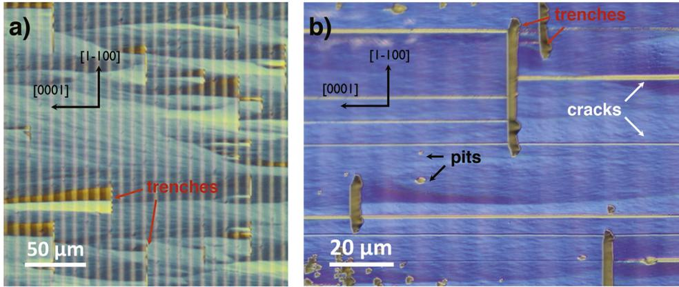
**Fig. 4.** Surface morphology of a) Sample D and b) Sample C by Nomarski interference light microscopy, showing trenches (uncoalesced regions during ELOG growth, indicated by the red arrows), cracks (marked as white arrows), and dislocation related surface pits (black arrows). (For interpretation of the references to colour in this figure legend, the reader is referred to the web version of this article.)
