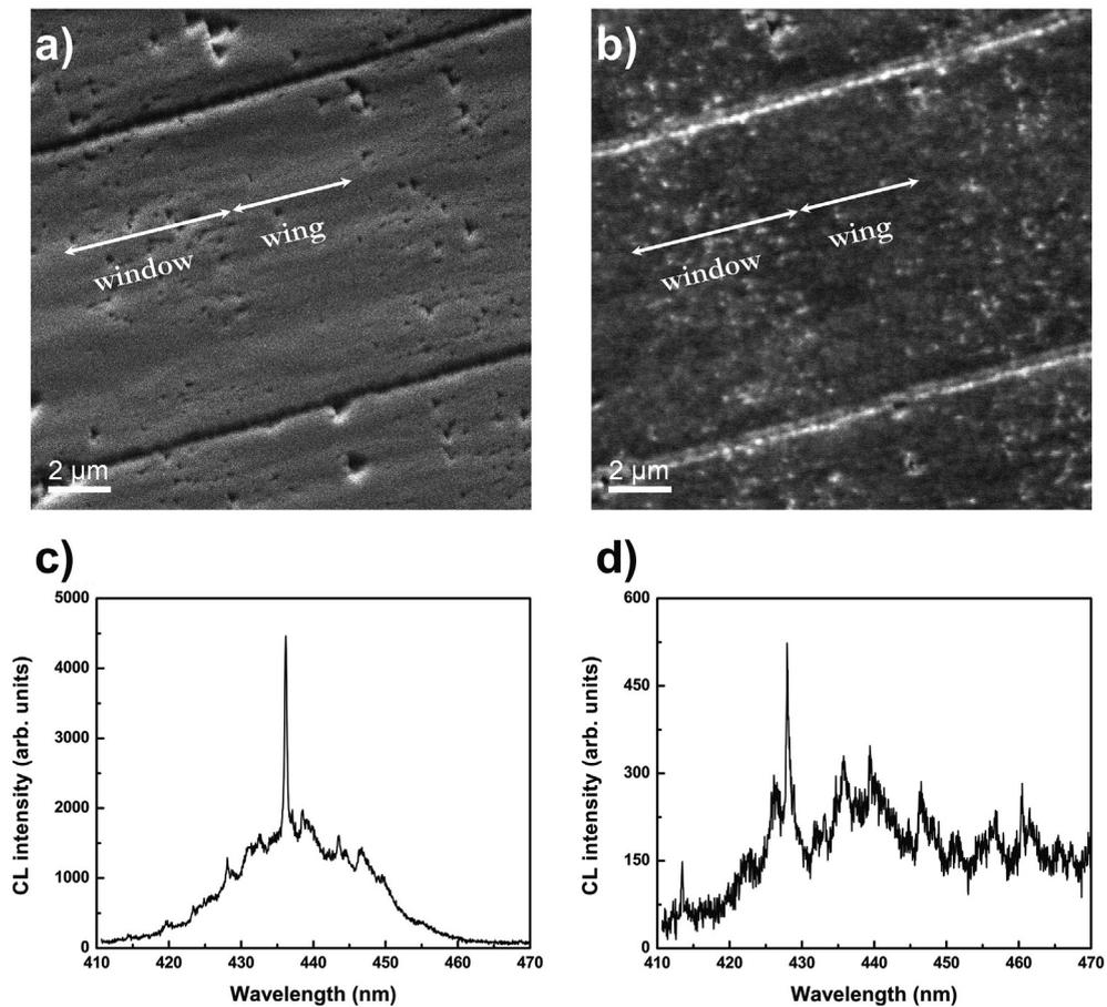
**Fig. 7.** a) SEM and b) panchromatic CL images of the capped QD sample with a 15-period AlN/GaN DBR (sample C). Typical CL spectra taken at 20 K from samples c) with DBR (sample C) and d) without a DBR (sample F) on ELOG pseudo-substrates.
