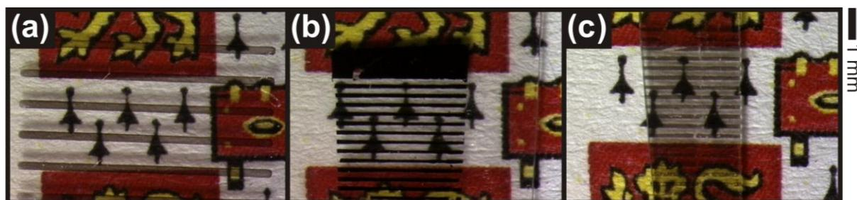
**Figure 4.4 | Transparency control and alignment.** (a-c) Optical micrographs of Mo-passivated patterned and dry-transferred MWCNT thin films on PET showing controllable transparency by adjusting the length of the source nanotubes.
