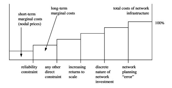
Figure 1: Cost drivers of a transmission network Source: Perez-Arriaga, 2003
