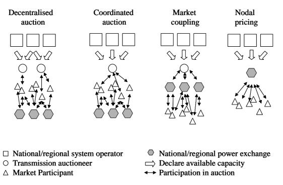
Figure 2: Different allocation mechanisms for scarce transmission capacity
