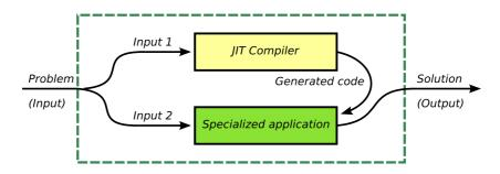
Fig. 2. An automated system (DOLFIN) using a JIT compiler (FFC or SyFi/SFC) to generate special purpose code for a subset of its input. For a typical finite element application, Input 1 consists of the variational problem and the finite element(s) used to define it, and Input 2 consists of the mesh.
