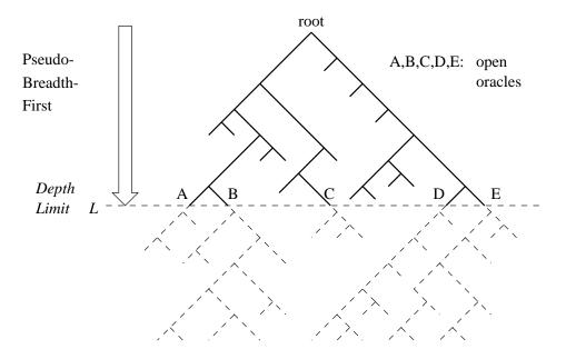
Figure 2.10: First phase of breadth-first partitioning.
