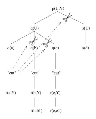
Figure 4.2: Effect of *cut* on OR-only search tree.
