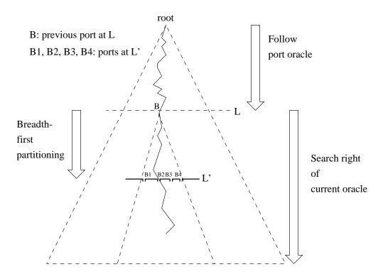
Figure 8.3: Assignment of work to an idle path processor.
