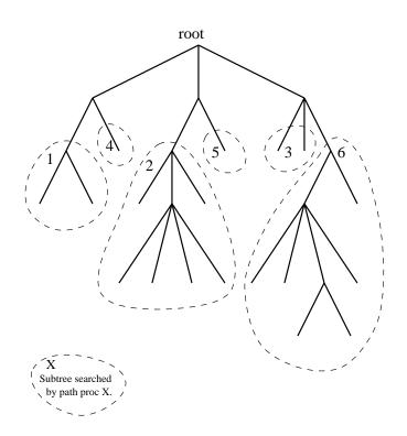
Figure 2.9: Partition central of sample tree in [49] for G = 6.
