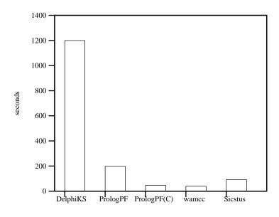
Figure 3.3: Single cpu runtimes for 10-queens benchmark.
