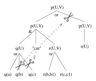
Figure 4.1: The effect of *cut* on the AND-OR search tree.
