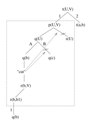
Figure 4.4: Deterministic execution of a PrologPF relation containing cut.
