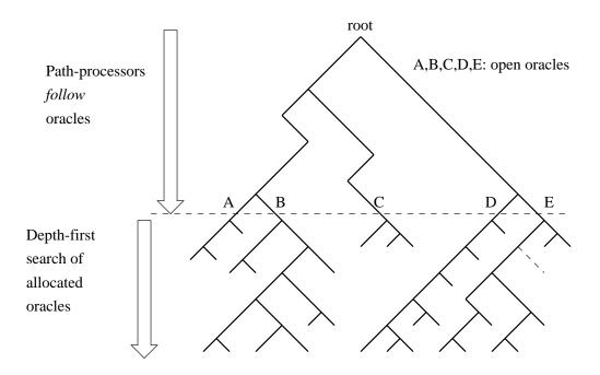
Figure 2.11: Second phase of breadth-first partitioning.
