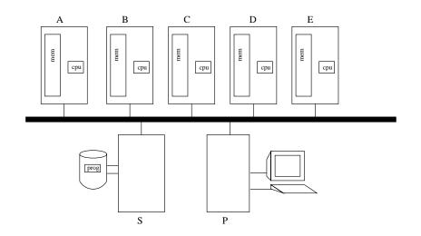
Figure 2.7: Distributed target architecture of the Delphi machine.
