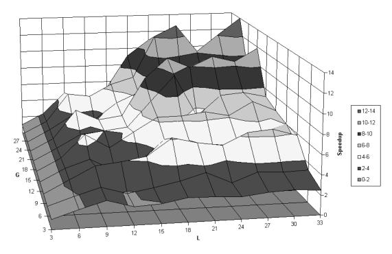
Figure 3.19: Speedup for Pentominoes benchmark for G = 1...30 and L = 1...33.
