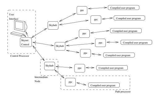
Figure A.1: System communications architecture
