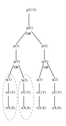
Figure 2.3: Variable bindings in OR-parallel subtrees.
