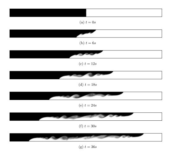
Figure A.13: Boussinesq half-depth gravity current evolution predicted by MO-BILE simulation,  $\rho_{\text{left}} = 1000 kgm^{-3}$ ,  $\rho_{\text{right}} = 1003 kgm^{-3}$ .
