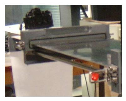
Figure 2.6: Detail of the barrier seal, an O-ring (coloured black) which seals two PVC blocks (coloured grey) held together with clips (coloured red) against hydrostatic pressure when the barrier is closed.
