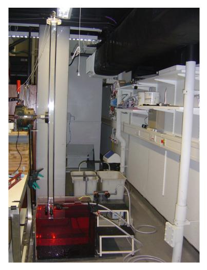
Figure 2.9: The high-aspect-ratio Rayleigh-Taylor instability experimental apparatus.
