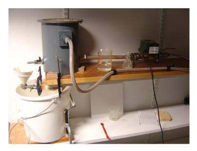
Figure 5.3: Recirculating pump, batch tank, output filter and settling bucket for production of saturated Acridine solution.
