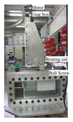
Figure 3.1 In-Flight Excavator
