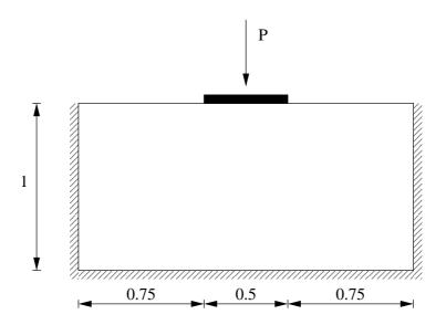
Figure 1: Plane strain punch test configuration. All dimensions in millimetres.
