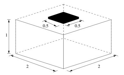
Figure 6: Three-dimensional punch test. The bottom and side surfaces of the prism are fully restrained and the infinitely stiff plate is located in the centre of the top surface. All dimensions in millimetres.
