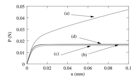
Figure 3: Load–displacement response for the plane strain punch test with (a) diagonal linear triangles, (b) crossed linear triangles, (c) diagonal quadratic triangles and (d) diagonal linear triangles with enhancement.
