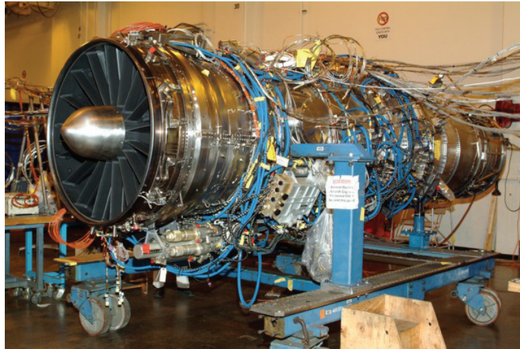
Figure 3.1 The GE Rolls-Royce Fighter Engine Team F136 turbofan engine (JSF, 2007).
