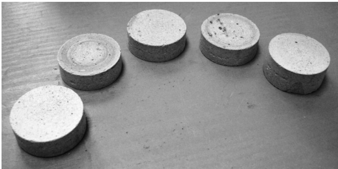
Figure 5.2: Photographs of permeability test specimens
