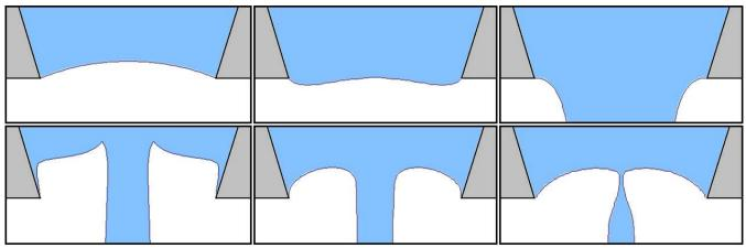
Figure 5. Fluid boundaries as calculated by Lagrangian simulations, times consistent with those at Figure 2. The unit of length is the nozzle radius d/2 = 40 µm.
