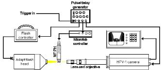
Figure 1. Schematic of the experimental arrangement used in this work.
