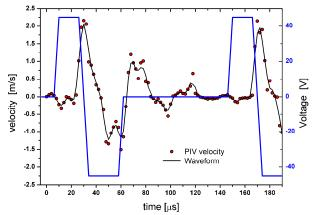
Figure 3. Time variation of the fluid velocity as measured by PIV. See Figure 2.
