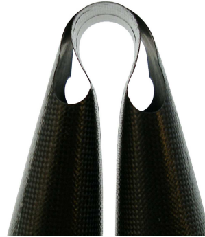
(c) Fully folded configuration (experiment)
