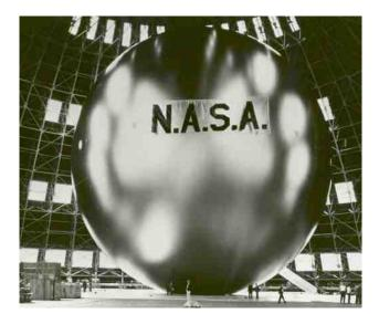
Figure 1.5: NASA's Echo II Balloon (which was rigidized when inflated).
