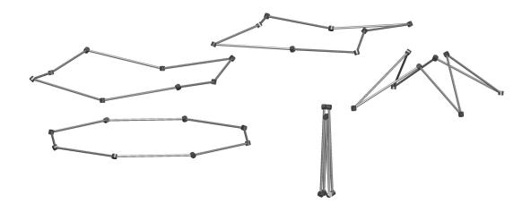
Figure 5.1: A doubly-symmetric 8-bar loop undergoing folding (clockwise from bottom left).
