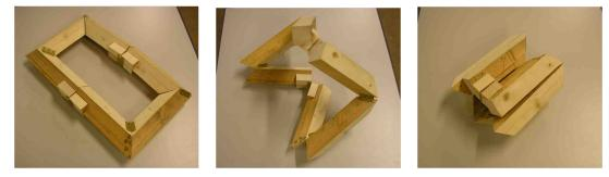
Figure 3.6: The folding of a wooden model with  $\alpha'_1 = \pi/4$ ,  $\alpha'_2 = -\pi/4$ , and hence  $\alpha_1 = \tan^{-1}(1/\sqrt{2})$ ,  $\alpha_2 = -\tan^{-1}(1/\sqrt{2})$ .
