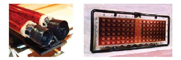
Figure 1.6: JPL's inflatable SAR frame. The flexible patch array and the inflatable booms are shown rolled up in the stowed state on the left.
