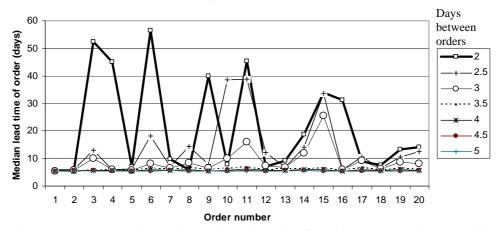
Figure 8 Median lead time for processing each of 20 consecutive orders, and variation in median lead times with the time between receiving orders
