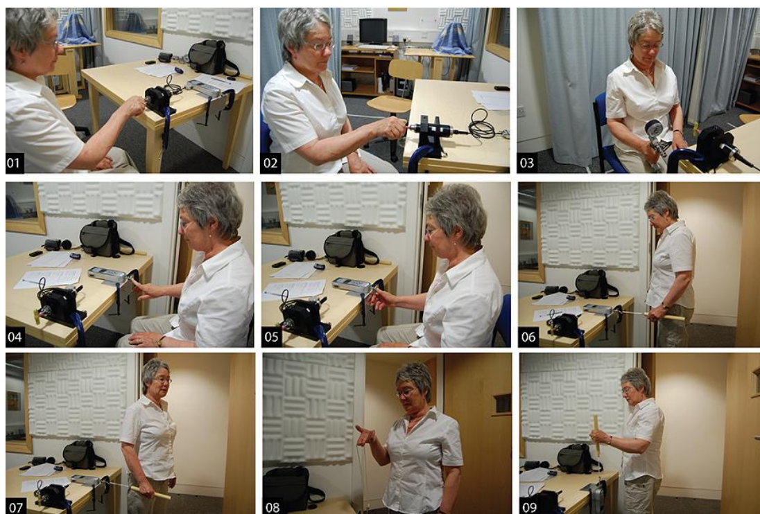
Figure 7-9 User performing motor capability tests: (01, 02) Twisting force measurement, (03) Grip strength measurement, (04, 05) Finger push force measurement, (06, 07) Pull and push force measurement, (08) Finger pull up force measurement and (09) Grasp and pull up force measurement.
