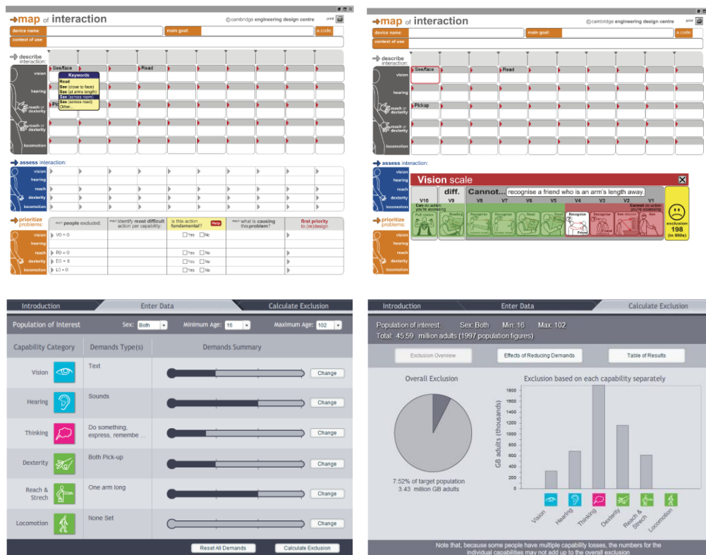
Figure 2-8 Exclusion audit tools showing interaction maps and an exclusion calculator based on the DFS capability scales
