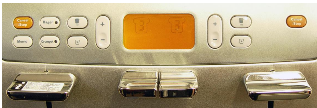
Figure 6-2 The interface of toaster 2 consisting of buttons, sliders and an LCD screen
