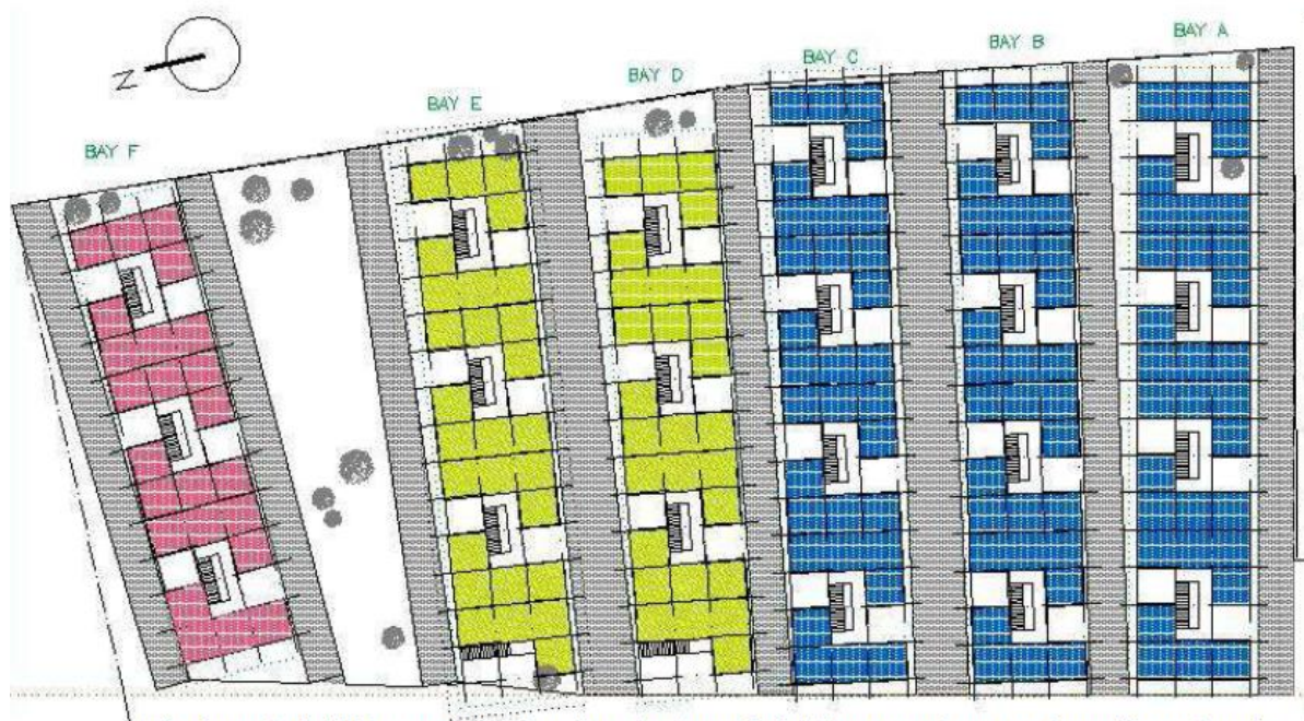
The layout of 176 tenements showing clusters of eight tenements around small courtyards.
