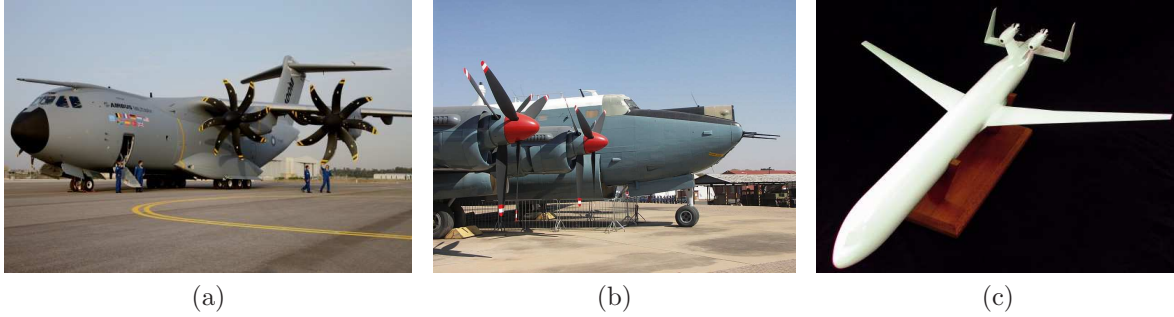
Figure 4.4: a) The Airbus A400m. b) The counter-rotating propellers of the Avro Shackleton. Photo by NJR ZA, licenced under Creative Commons Licence. c) Example of the rear mounted AOR concept being developed by Airbus.
