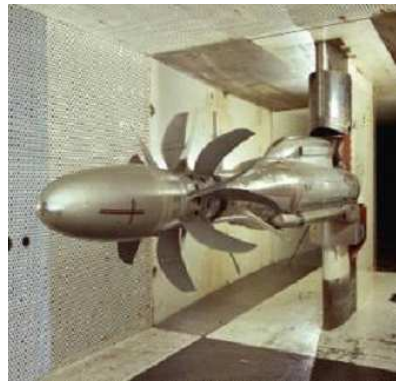
Figure 3.9: The large ‘bullet’ protruding upstream of the rotors in Rig 140 testing in the 1980s. Reproduced with permission from Rolls-Royce.
