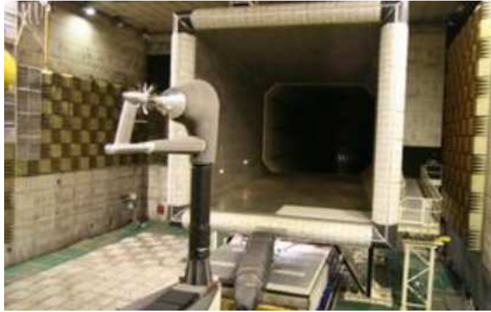
Figure 4.1: Rig 145 testing between 2008-2010 included measurements with the pylon in place. Image reproduced with permission from Rolls-Royce. The pylon of an open rotor must be substantial in order to withstand blade-off failure testing.
