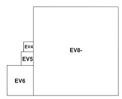
Figure 2.2: Size comparison of a set of DEC Alpha cores from a heterogeneous multicore chip; each core is labelled with the single-core chip in which it originally appeared. Reproduced from [Kumar et al., 2003].
