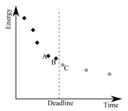
Figure 5.3: An example set of operating points and a per-frame deadline shown in energy—time space.
