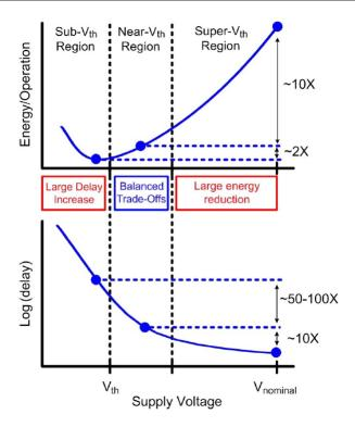
Figure 2.4: Transistor behaviour in sub-, near-, and super-threshold operating voltage regions. Reproduced from [Dreslinski et al., 2010].
