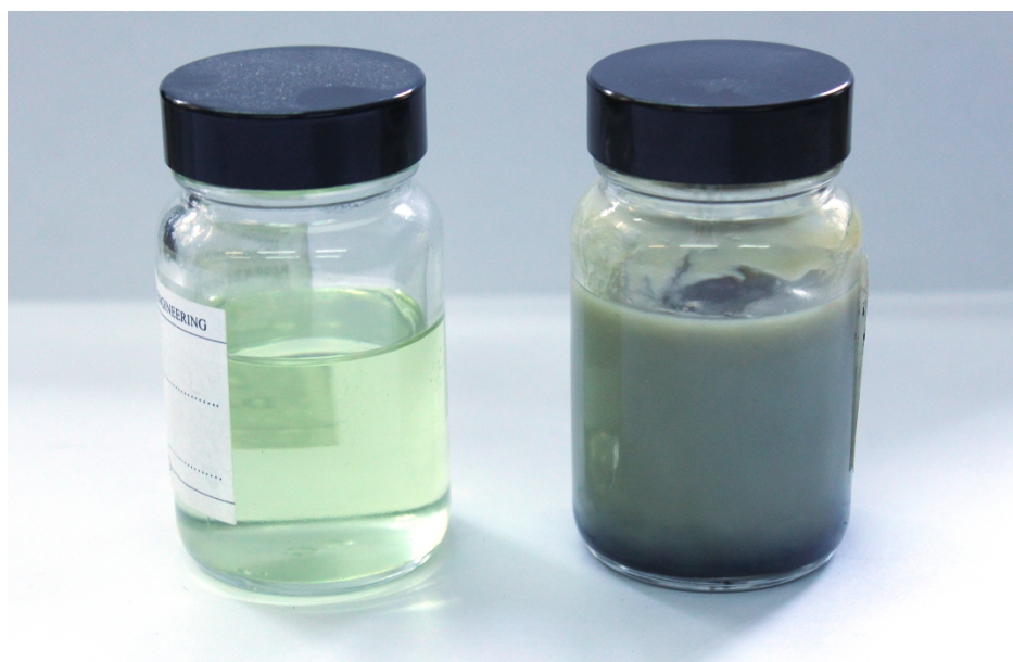
Figure 4.1: Condensed pyrolysis products generated using activated carbon (left) and coke (right) reactor beds. The activated carbon derived condensate is entirely liquid at room temperature and clear — notice that it is sufficiently transparent that the sample label is clearly visible at the rear of the glass sample bottle. The condensate produced using a coke bed, by contrast, is mostly solid at room temperature and entirely opaque.
