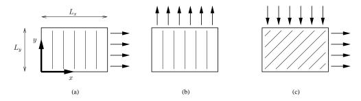
Figure 11: Rectangular membrane test cases for extraction of engineering constants from the FE material representation: (a) pure longitudinal strain; (b) pure lateral strain; and (c) pure shear strain on  $45^{\circ}/135^{\circ}$  planes. Lines inside rectangles indicate the reinforcement direction for each case.
