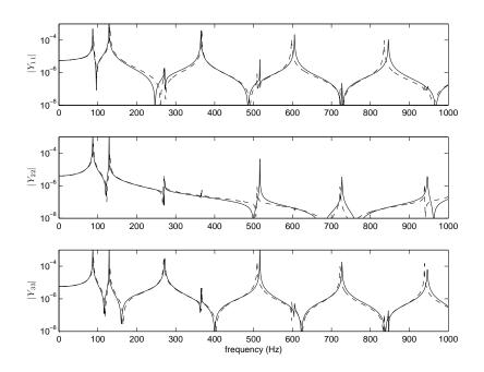
Figure 16: Diagonal admittance components for the uniform (—) and varying thickness (– –) sidewalls. Azimuthal order n = 2.
