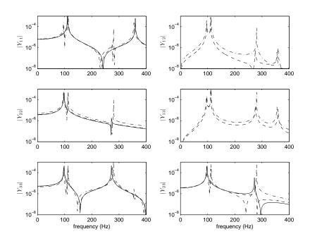
Figure 17: Influence of rotation on n = 0 admittance components for the uniform sidewall. —: 0 km/hour; - -: 130 km/hour; --: 260km/hour
