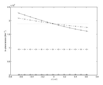
Figure 5: In-plane tensions for the non-rotating case: —, FE calculation; – –, analytical solution for torus. Azimuthal components are indicated by circular markers, and meridional by crosses. Also shown is a dotted line at the value of  $pR_s$ .
