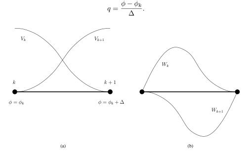
Figure C.19: The basis functions associated with the kth element, which lies between nodes k and k + 1. (a)  $V_k(\phi)$  and  $V_{k+1}(\phi)$ ; (b)  $W_k(\phi)$  and  $W_{k+1}(\phi)$ .
