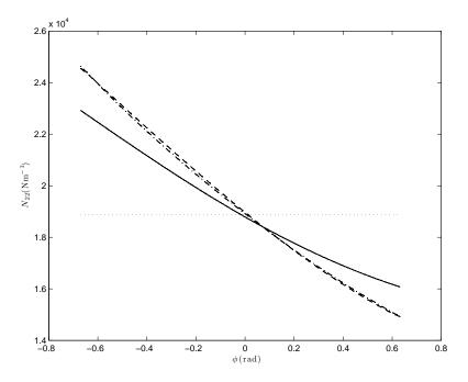
Figure 6: Meridional tensions for: —, non-rotating case; – –, uniform-thickness rotating case; ––, varying thickness rotating case. Dotted line at  $pR_s$ .
