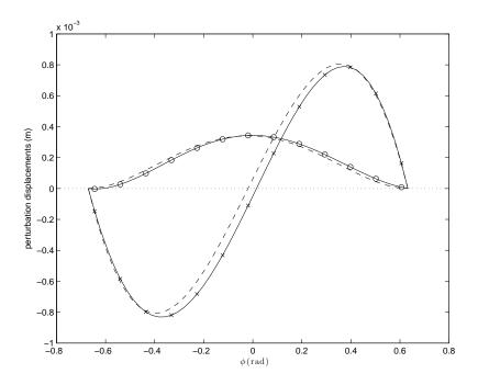
Figure 8: Displacements relative to equivalent circular arc for uniform-thickness rotating case: —, FE calculation; – –, approximate solution. Circular markers indicate tangential component,  $w_{\phi}$ ; crosses normal component,  $w_n$ .
