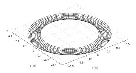
Figure 2: Finite-Element mesh topology. This (low-resolution) example consists of 100 (azimuthal)  $\times$  10 (meridional) quadrilateral elements, with uniform angular spacing in each direction.
