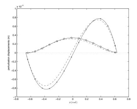
Figure 9: Displacements relative to equivalent circular arc for varying thickness rotating case: —, FE calculation; – –, approximate solution. Circular markers indicate tangential component,  $w_{\phi}$ ; crosses normal component,  $w_n$ .
