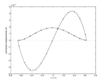
Figure 7: Displacements relative to equivalent circular arc for non-rotating case: —, FE calculation; – –, approximate solution. Circular markers indicate tangential component,  $w_{\phi}$ ; crosses normal component,  $w_n$ .
