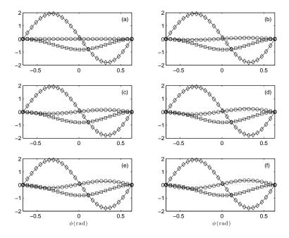
Figure 13: Displacement amplitudes in the uniform-sidewall second mode at azimuthal orders 0 (a) to 5 (f). Legend as Fig. 12.
