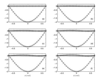
Figure 12: Displacement amplitudes in the uniform-sidewall first mode at azimuthal orders 0 (a) to 5 (f). Lines show results from current model, symbols those from FE (subsampled for clarity). o:  $\text{Im}(u_1^{kn})$ ;  $\Box$ :  $\text{Re}(u_2^{kn})$ ;  $\Diamond$ :  $\text{Re}(u_3^{kn})$ . Note that  $\text{Re}(u_1^{kn}) = \text{Im}(u_2^{kn}) = 0$ .
