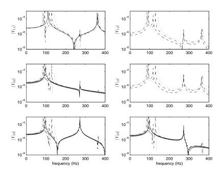
Figure 14: Admittance components for the uniform sidewall. —: n = 0; - -: n = 1; ---: n = 2; ...: n = 3; •: one-dimensional model ( $Y_{22}$ ,  $Y_{33}$  and  $Y_{23}$  only).
