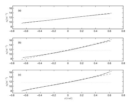
Figure A.18: Meridional curvatures for (a) uniform-thickness, non-rotating; (b) uniform-thickness, rotating; and (c) varying thickness, rotating cases. Comparisons are between FE results (—), analytical approximations (– –) and values derived from the analytical approximation to  $N_{22}$  (––). Dotted lines at  $1/R_s$ .
