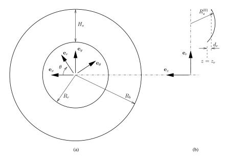
Figure 1: The unloaded sidewall geometry: (a) side view; (b) cross-sectional view. The shape is toroidal, with circular edges of radius  $R_r$  and  $R_b$ . The inner edge is offset from the outer by a distance  $d_r$ , and the cross-sectional arc radius is  $R_s^{(0)}$ . Cartesian and rectangular-polar coordinate systems are defined by their respective unit vectors.
