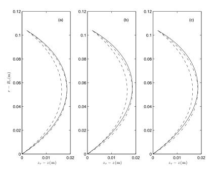
Figure 3: Loaded sidewall shapes for: (a) uniform thickness, non-rotating; (b) uniform thickness, rotating; and (c) varying thickness, rotating cases. Included for comparison are the unloaded shape (--) and the 'equivalent circular arc' with length equal to the loaded shape (--). Axes are chosen for consistency with the cross-sectional view in Fig. 1(b).
