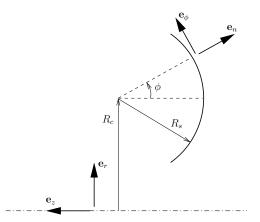
Figure 4: Local coordinate system based on the equivalent circular arc (of radius  $R_s$ .) The parameter  $R_c$  is the distance from the tyre axis to the arc's centre.
