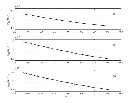
Figure 10: Meridional tensions for (a) uniform-thickness, non-rotating; (b) uniform-thickness, rotating; and (c) varying thickness, rotating cases. Comparisons are between FE results (—) and analytical approximations (– –). Dotted lines at  $pR_s$ .
