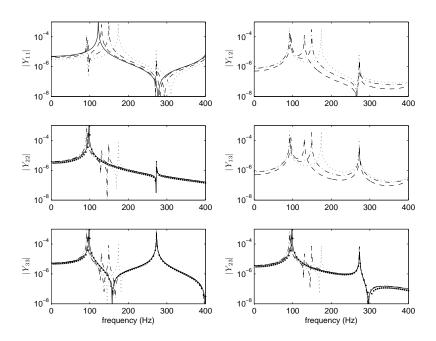
Figure 15: Admittance components for the uniform sidewall with dynamically stiffened rubber modulus. —: n = 0; - -: n = 1; --: n = 2; ...: n = 3; •: one-dimensional model ( $Y_{22}$ ,  $Y_{33}$  and  $Y_{23}$  only).
