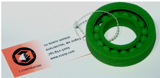
FIG. 9: (Colour online) Example of a rapid prototyping process; a bearing printed by the Z-Corp process using non-functional materials.
