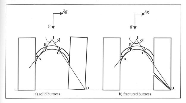
*Figure 7.7* Collapse mechanisms for buttressed arches under horizontal acceleration. The instantaneous centre, I, of the central portion can be used to calculate the relative rotation of each segment.
