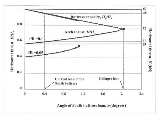
*Figure 8.3* Changing horizontal thrust as the South buttress leans for the church at Goa. Collapse occurs when the buttress leans by just over  $2^{\circ}$ , and the thrust of the deformed arch exceeds the capacity of the leaning buttress. If the arch were half the thickness (t/R = 0.05), then the arch would collapse before exceeding the buttress capacity, at a buttress lean of  $1.1^{\circ}$  (shown by the lowest curve).
