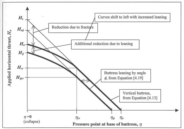
*Figure 4.8.* Influence of leaning on buttress reaction and capacity. The pressure point at the base of the buttress moves toward the edge as the horizontal load is increased. The presence of buttress leaning shifts the entire curve to the left.
