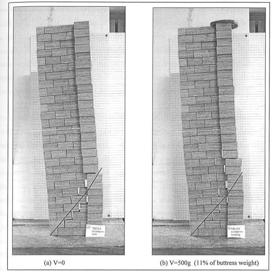
*Figure 3.11* Test on T-shaped buttress with  $h_t/b=4$  and  $\mu=0.5$  with a solid line for the predicted fracture. The horizontal load is applied from the left by the white string, and the buttress is shown in the post-collapse configuration after it has reached its maximum capacity.
