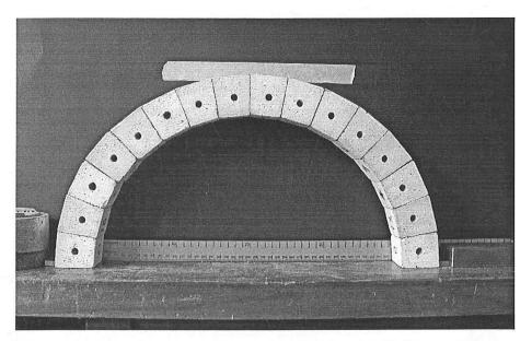
Figure 5.18. Undeformed masonry arch of approximately 11° blocks (Arch1: t/R=0.23,  $\alpha=90^{\circ}$ ).
