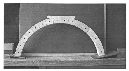
Figure 5.20. Undeformed masonry arch of 10° blocks (Arch2: t/R=0.13, a=80°).
