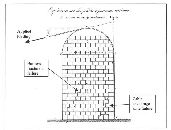
**Figure 2.2** Experiment on masonry pier for a suspension bridge showing fracture at collapse (Vicat 1832). The cable "pulls" the buttress over in the same way that a horizontal thrust from an arch or vault would "push" against the buttress.
