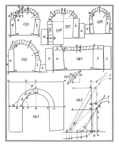
*Figure 1.2* Collapse mechanisms in masonry arches from experiments by Danyzy in 1732 (Heyman 1995).
