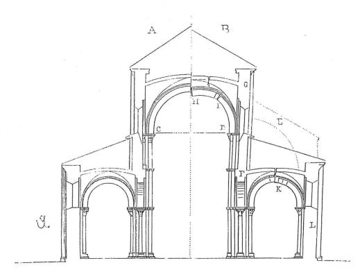
*Figure 2.10* Deformed state of the Church at Vézelay, France (Viollet-le-Duc 1854). On the left as originally designed, and on the right as distorted.
