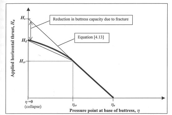
Figure 4.7. Movement of pressure point at base of buttress as horizontal thrust is increased (see Fig. 4.6.)
