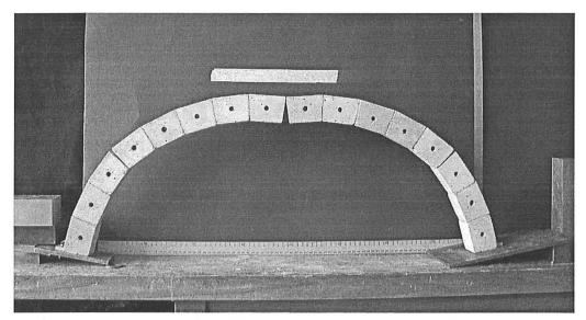
Figure 5.21. Deformed Arch2 on spreading supports just before collapse.
