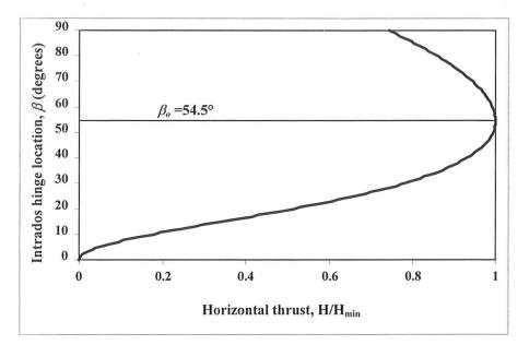
*Figure 5.9.* Horizontal thrust from the central region (ABC) of a semi-circular arch with t/R = 0.1075 as a function of the location of the intrados hinge  $\beta$ . Not all hinge locations are statically admissible, but the maximum value will correspond to the correct hinge location for the state of minimum thrust. This curve corresponds to the thrust from equation [5.3] for a circular arch, and is normalised by the correct value of minimum thrust,  $H_{min}$ .
