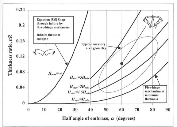
*Figure 5.12.* Collapse mechanisms and associated horizontal thrust for circular arches on spreading supports. The maximum horizontal thrust from the arch at collapse is defined as  $H_{max}$ , a multiple of  $H_{min}$ .
