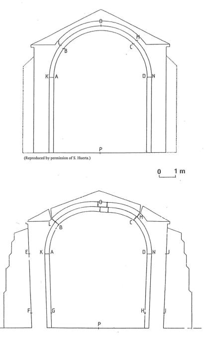
*Figure 1.1* Severe deformations in a barrel vault, Guimarei, Spain (Huerta and López 1997). The upper diagram shows the church as built, with buttresses of uniform thickness. The lower diagram shows the current conformation, in which the outer stepped buttresses were added later in an attempt to reinforce the severely deformed church.
