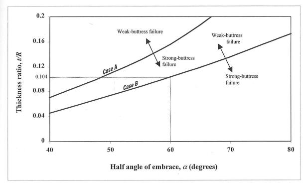
*Figure 7.6* Minimum thickness for the thrust of the deformed arch to exceed the capacity of the leaning buttress, i.e. threshold thickness between "weak-buttress" and "strong-buttress" failure. For example, an arch subtending  $120^{\circ}$  ( $\alpha$ =60°) will fail by weak-buttress collapse when the thickness ratio is greater than t/R = 0.104.
