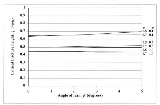
*Figure 4.3* Variation in fracture height for a leaning rectangular buttress  $(h_b/b=4)$ .
