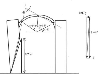
*Figure 8.9.* If the South buttress is assumed to fracture as predicted under a constant vertical load and an increasing horizontal load, the church will collapse for a lower value of horizontal acceleration. As before, three hinges would form in the arch at the collapse state, though the reduced buttress mass would lower the threshold acceleration to 0.07g.
