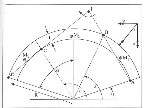
Figure 6.2. Geometry of a circular masonry arch with four hinges due to horizontal acceleration.
