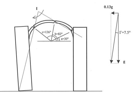
*Figure 8.8.* Collapse state of the church at Goa due to constant horizontal acceleration of 0.13g. The South buttress is assumed to remain solid, and three hinges form in the arch at the collapse state. The collapse state has been determined using the program SolidTilt, and the structure has been analysed in its undeformed state using work calculations based on an infinitesimal motion.
