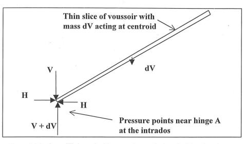
Figure 5.3 Static equilibrium of a thin voussoir near the intrados hinge location.
