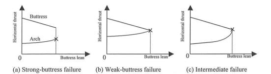
*Figure 8.5.* Three types of failure for an arch supported on leaning buttresses. The horizontal axis presents the inclination of the buttress and the vertical axis presents the change in horizontal thrust as the buttresses lean outwards. The arch collapse state is marked by "x".
