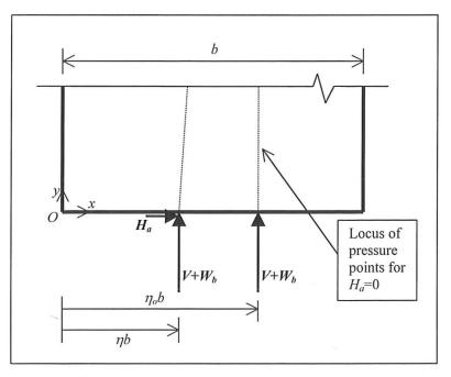
*Figure 4.6.* Reaction point,  $\eta b$ , at the base of the buttress for an applied horizontal thrust,  $H_a$ . The thrust is applied from the right, and the vertical load, V, is applied at the right-hand edge. If no horizontal thrust is applied ( $H_a = 0$ ), the reaction point occurs at the resultant of the vertical loads,  $\eta_a b$ . The origin is defined as the point O about which overturning may occur.
