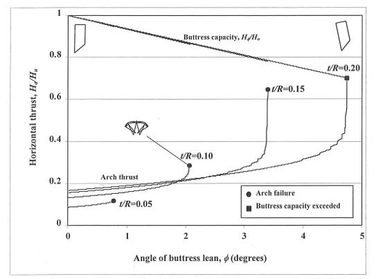
*Figure 7.3* Collapse state for buttressed arch Case A due to leaning buttresses ( $\alpha$ =60°). The problem is analysed using the program ArchLean, for an arch constructed of 1° voussoirs in each case.
