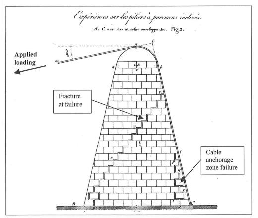
*Figure 4.1* Experiments on masonry towers for suspension bridges (Vicat 1832). As in Figure 2.2, the tower served as the anchorage for the cable, which extended around the top of the tower. The applied load is equivalent to an inclined load at the top of the tower, similar to the thrust of a vault, where the load of the cable applies both a vertical and horizontal load to the top of the tower.
