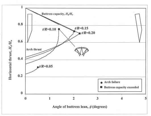
*Figure 7.4* Collapse state for buttressed arch Case B due to leaning buttresses ( $\alpha = 60^{\circ}$ ). The problem is analysed using the program ArchLean, for an arch constructed of 1° voussoirs in each case.
