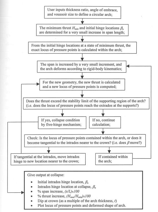
*Figure 5.11* Algorithm to determine the collapse state of an arch on spreading supports.
