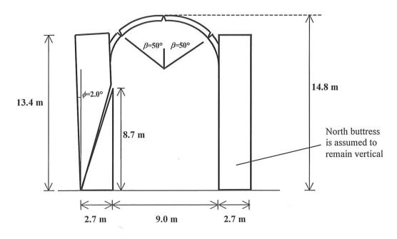
*Figure 8.2.* Collapse state of the church at Goa due to leaning of the South buttress. When the buttress has leaned outward by  $2^{\circ}$ , the thrust from the distorted vault will exceed the thrust capacity of the buttress and the vault will collapse. At this point, the crown of the vault has descended by 0.4 m and the thrust of the arch will have increased from 41 kN to 52 kN.
