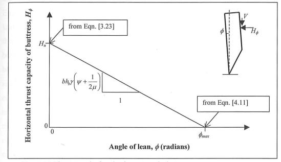
Figure 4.5 Thrust capacity for a leaning rectangular buttress.
