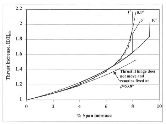
Figure 5.17. Thrust increase with span increase for various voussoir sizes ( $\alpha$ =60°, t/R=0.10).
