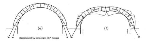
*Figure 2.11* "Kinematic" safety factor for an arch on spreading supports (Smars 2000). The image on the left illustrates the minimum and maximum states of horizontal thrust for the arch as originally constructed. The image on the right is the arch at a possible collapse state due to spreading supports.
