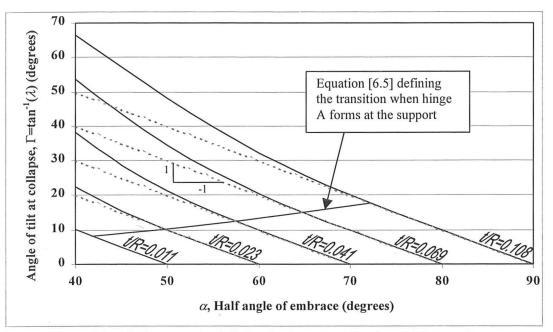
Figure 6.5. Maximum angle of tilt for circular arches of various thickness ratios.
