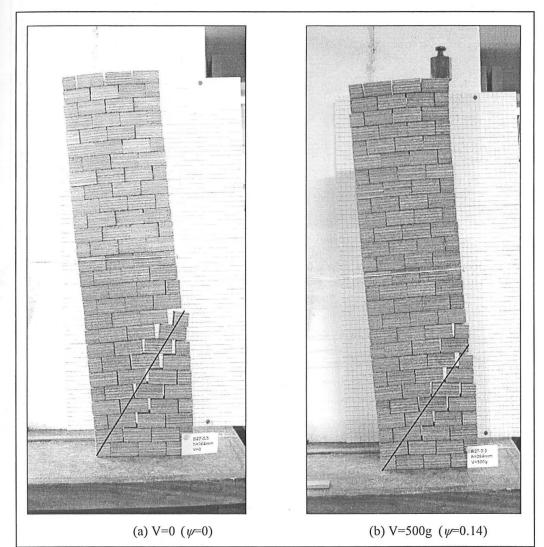
**Figure 3.10.** Test on rectangular buttress with  $h_b/b=4$  and  $\mu=0.5$  with a solid line for the fracture predicted by the method of section 3.6. The horizontal load is applied from the left by the white string, and the buttress is shown in the post-collapse configuration after it has reached its maximum capacity.
