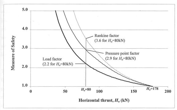
*Figure 4.9.* Safety factors for the rectangular buttress example from Chapter 3.  $(h_b=12 \text{ m}, b=3 \text{ m}, h=8 \text{ m}, \gamma=29.4 \text{ kn/m}^2, V=100 \text{ kN}, H_{cr}=91 \text{ kN}, H_u=178 \text{ kN})$
