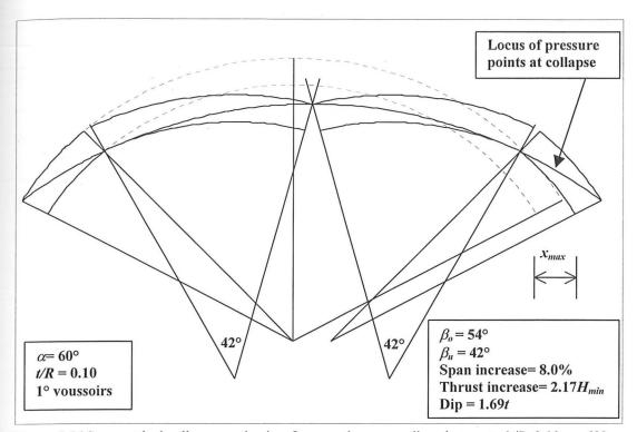
*Figure 5.16* Symmetrical collapse mechanism for an arch on spreading abutments (t/R=0.10;  $\alpha=60^{\circ}$ ; voussoir angle =1°).
