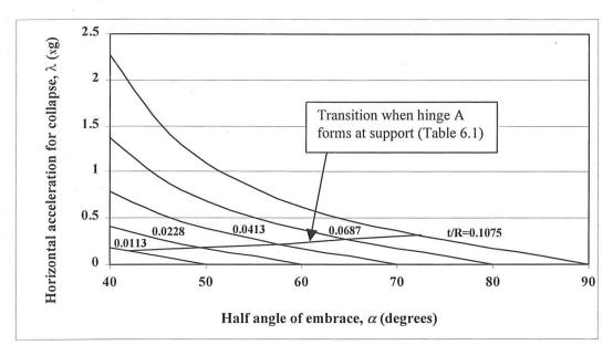
*Figure 6.6* Value of horizontal acceleration for collapse of a circular arch. The simple approximation described in this chapter is tangent to each curve for small values of acceleration, as in Figure 6.5.
