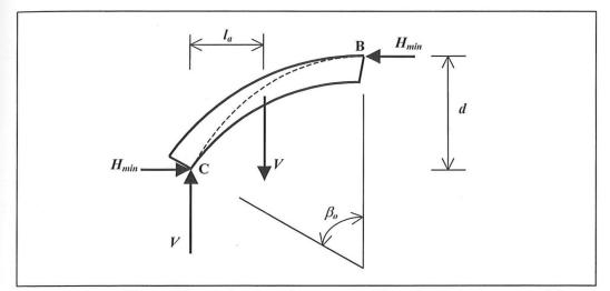
*Figure 5.8.* Equilibrium of central region of a masonry arch, acting under its own weight, at the state of minimum thrust,  $H_{min}$ , due to a very small outward movement of the supports. The arch is symmetrical, so this analysis can be applied to section BC or section AB of the arch.
