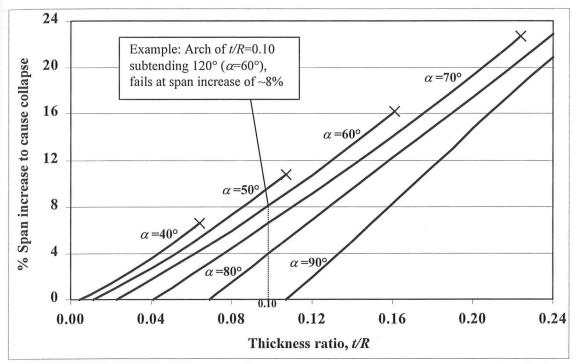
*Figure 5.14* Maximum span increase at collapse for circular arches. Some plots are terminated when the thrust of the arch at collapse is equal to five times the minimum thrust. These points are marked by "x" and correspond to the same points on Figure 5.13.
