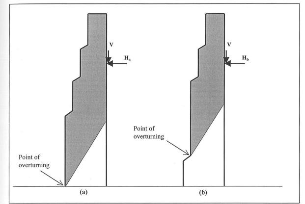
*Figure 3.7.* Possible fracture patterns in various Gothic buttresses at the point of overturning due to an applied horizontal thrust, *H*. The shaded areas represent the effective mass of each buttress that contributes to the stabilising moment to resist the applied horizontal load.
