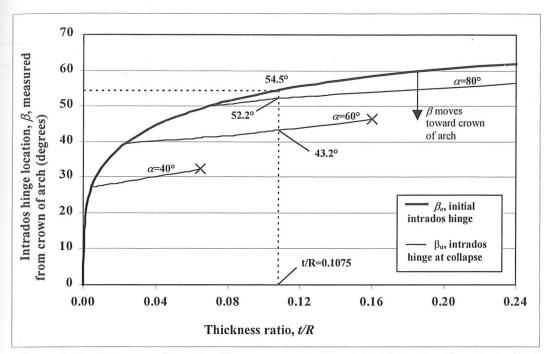
*Figure 5.15.* Summary of intrados hinge movements from initial hinge location,  $\beta_o$ , to final hinge location at the collapse state,  $\beta_u$ , assuming the voussoir size is 0.1°.
