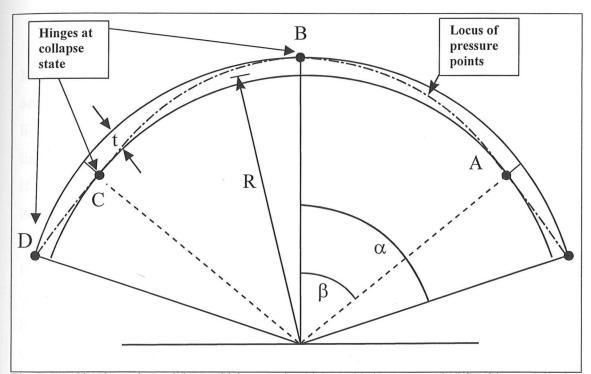
**Figure 5.2** Circular arch at minimum thickness ratio,  $(t/R)_{min}$ . This is a symmetrical five-hinge mechanism, though in practice, slight asymmetries will exist and four hinges are sufficient for collapse. The four-hinge collapse mechanism must have hinge rotations of alternating sign in order to be kinematically admissible.
