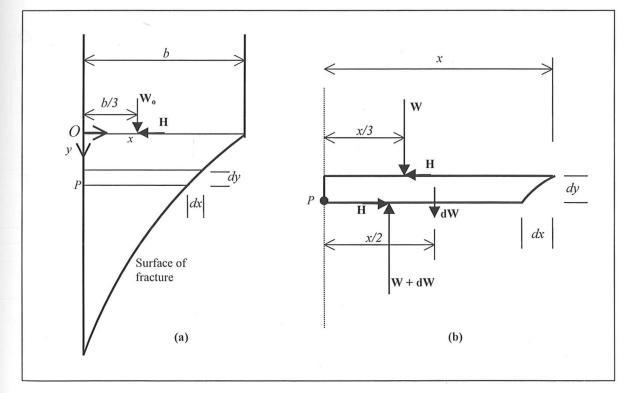
*Figure 3.3.* (a) Equilibrium in the lower fractured region of the buttress; (b) Equilibrium of a horizontal slice. The horizontal force, H, is applied from the right, and overturning is assumed to occur about the lower left corner. The origin O of a cartesian (x, y) co-ordinate system is shown in (a), where the fracture begins.
