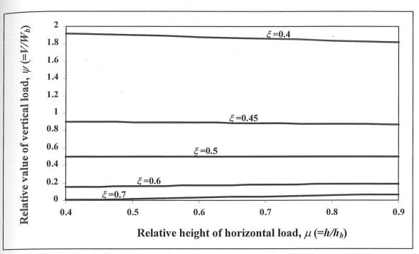
Figure 3.5. Variation in fracture height,  $\xi$ , as determined from Equation [3.25] for rectangular buttresses.
