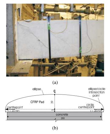
**Figure 5.** (a) Photo of 150 mm wide concrete beam with top and bottom steel support pads and (b) possible support pad geometry for 260 mm wide beam
