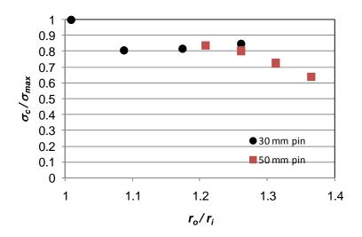
Figure 3. Non-laminated pin-loaded strap experimental results (Winistörfer et al 2001)
