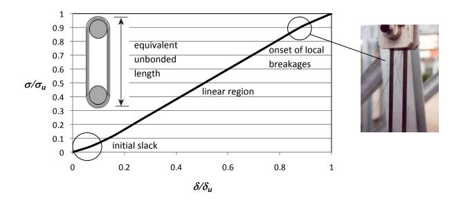
Figure 7. – Schematic strap load-displacement behaviour
