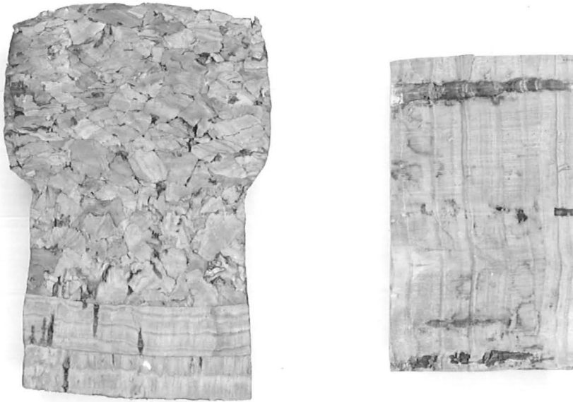
Fig. 7.13 A section through a champagne cork, and through a normal cork.
