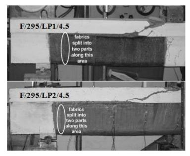
Fig. 6–F/295/LP1/4.5 and F/295/LP2/4.5 at failure.
