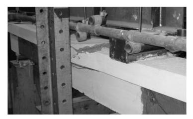
Fig. 8–Flexural failure of F/295/LP1/3.3.
