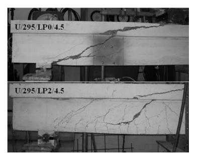
Fig. 5–Unstrengthened specimens at failure.
