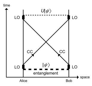
Figure 1.4: In an instantaneous nonlocal quantum computation, a given nonlocal unitary U is applied to a distributed quantum state  $|\psi\rangle$  after a single round of classical communication (CC) between the parties (Alice and Bob) sharing the state. The protocol consists of local operations (LO), which include measurements, on  $|\psi\rangle$  and shared entanglement, communication of the measurement results and further local operations.
