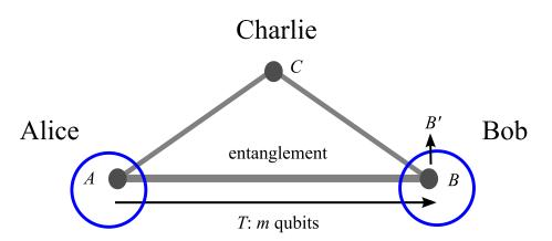
Figure 4.2: Setting for quantum information causality. Alice, Bob and Charlie have respective quantum systems A, B and C in an arbitrary quantum state, which can be entangled in any possible way. After applying local operations on her system, Alice obtains a quantum system T of m qubits that she sends Bob. Bob receives T and applies local operations on the system BT, which is denoted as B' after Bob's operations.
