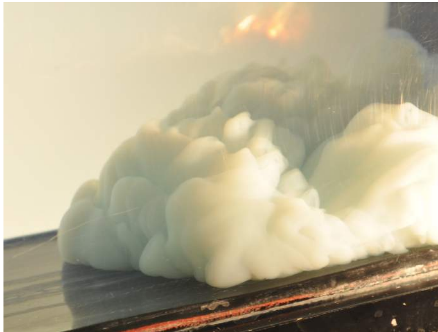
FIGURE 4.7: Photograph of the head of a turbulent gravity current as it flows from right to left.
