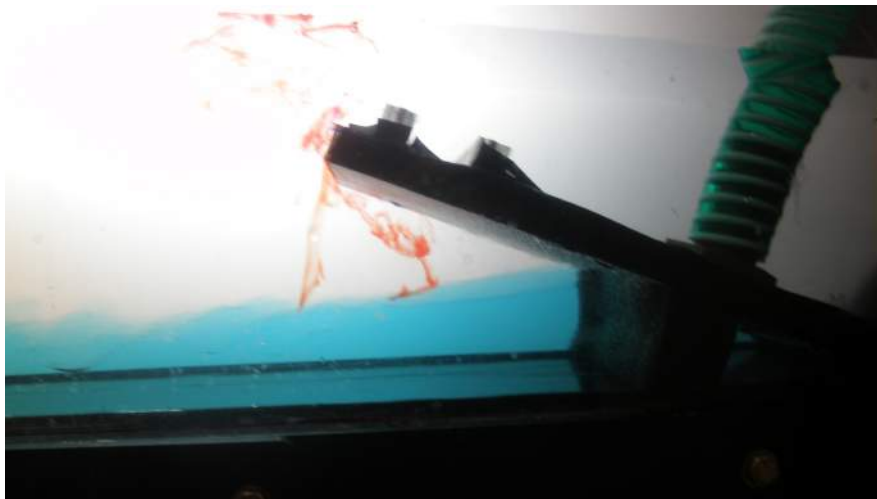
FIGURE 4.5: Photograph of red dye pipetted into the ambient fluid at the upper, downstream edge of the source unit. There is relatively little shear or turbulence in the ambient fluid above the gravity current. Strong shear and dilution is visible at the turbulent interface of the current. The deformation of the fluid filament observed above the source unit was caused by removing the pipette.
