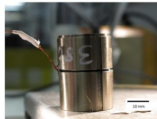
**Figure 1.** The assembled stack of two GdBCO bulk samples, each 24.15 mm in diameter and 15 mm high. The samples were reinforced with a 3 mm thick ring fabricated from 304 Stainless Steel. The recess visible in the ring served to accommodate the measurement wiring. The two bulk samples were then assembled into a stack with an array of five Hall probes at their interface using STYCAST thermally conductive epoxy resin. The Hall probes were arranged
