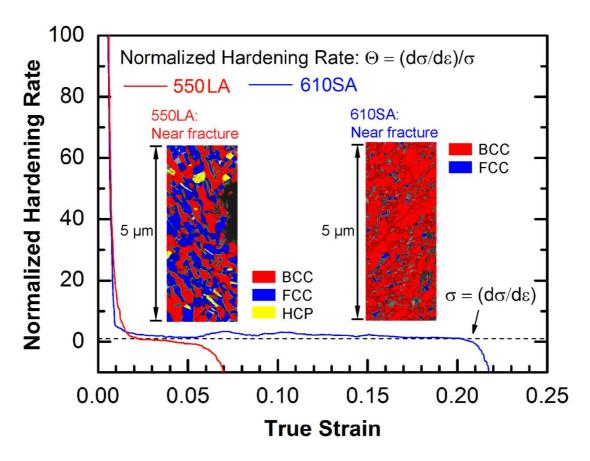
Figure 12 The change in normalized strain hardening rate with true strain and the TKD phase maps near the fracture surface of the 550LA and the 610SA steels. The black dashed line indicates the limit of plastic instability.
