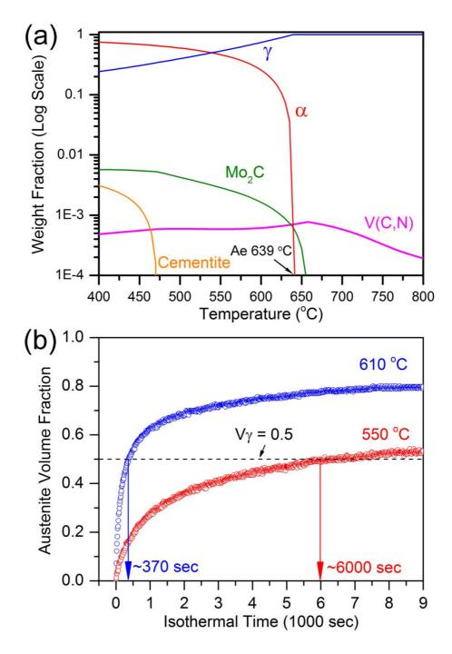
Figure 1 (a) The equilibrium phase fractions of the alloys at different temperature, computed using Thermo-Calc with the TCFE7 database, and (b) the volume fractions of austenite as a function of isothermal transformation time at 610 °C and 550 °C, measured using dilatometry.
