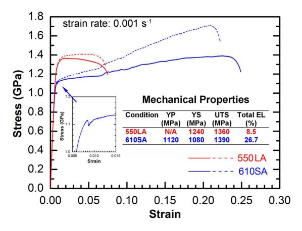
Figure 5 The engineering stress-strain curves (solid lines) and true stress-strain curves (dash lines) of the 550LA and 610SA steels.
