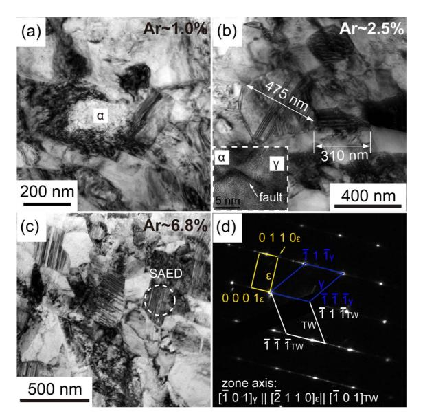
Figure 8 TEM bright field images revealing the deformation-induced microstructure in the 550LA steel strained by (a) ~1.0 %, (b) ~2.5%, and (c) ~6.8%, and (d) the corresponding electron diffraction analysis from the selected area in (c). These strain percentages relate to the percent reduction in cross-sectional area, Ar, during the uniaxial tensile test.
