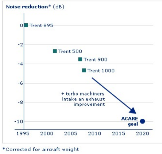
Figure 0.1: Aeroengine noise reduction over time due to improving designs. Source: Rolls-Royce.
