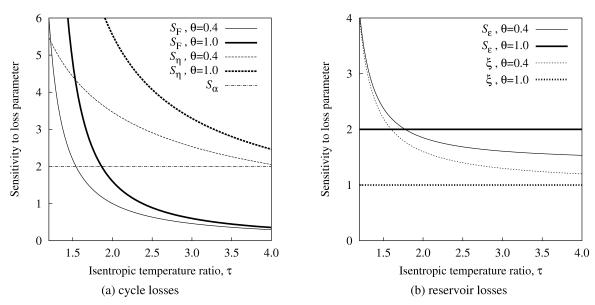
Figure 5: Variation of the loss sensitivity factors with isentropic temperature ratio for  $\theta$ =1 (bold) and  $\theta$ =0.4 (faint). Note that the  $\xi$  curves (right-hand figure) are with k=1/2.
