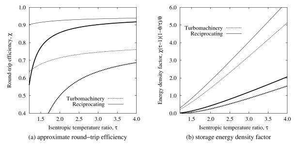
Figure 2: Approximate round-trip efficiency and energy density for  $\theta$ =1 (bold) and  $\theta$ =0.4 (faint)
