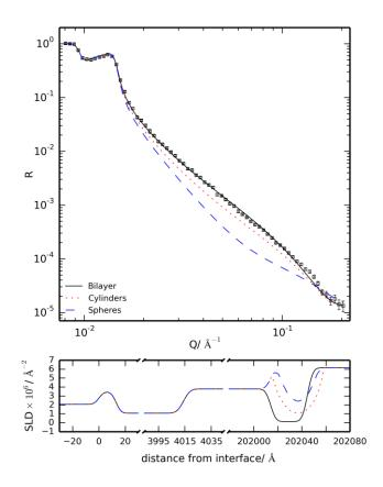
**Figure 5** [top] Data collected for the bare surface and  $C_{16}TAB$  layer at 1 CMC in  $D_2O$  along with fits to the data attempted using models for a bilayer, cylindrical micelles and spherical micelles. [bottom] SLD profiles extracted from fits.
