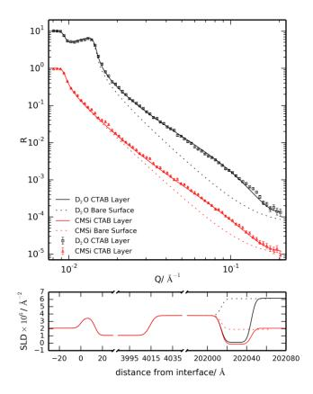
**Figure 3** [top] Measured reflectivity profiles and fits to data plotted on a log-log scale. Fits for the bare surface are shown for comparison as dashed lines. D<sub>2</sub>O contrasts are shown as squares and contrast matched to silicon (CMSi) contrasts as triangles. D<sub>2</sub>O data and fit have been offset by a factor of ten for clarity. [bottom] SLD profiles extracted from fits.
