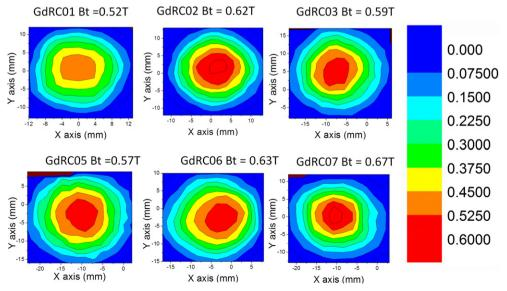
Fig. 4. Contour maps of the trapped field, B<sub>t</sub>, of recycled Gd-Ba-Cu-O-Ag samples.
