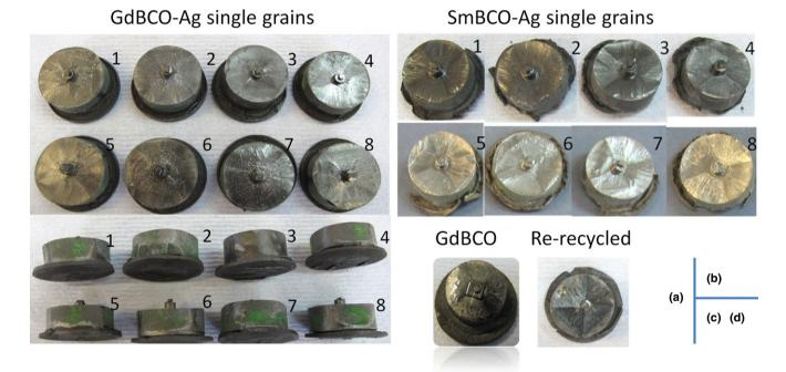
**Fig. 3.** Recycled (RE) -Ba-Cu-O-Ag (RE: Y, Gd, Sm) single grains (a) top and side views of one batch of 8 recycled Gd-Ba-Cu-O-Ag single grains 25 mm in diameter (b) top views of 8 Sm-Ba-Cu-O-Ag single grains 25 mm in diameter (c) top view of a recycled Gd-Ba-Cu-O single grain 20 mm in diameter (d) top view of re-recycled Y-Ba-Cu-O single grain 25 mm in diameter.
