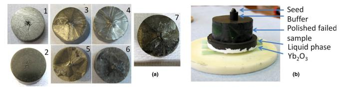
Fig. 1. Procedure for recycling failed Y-Ba-Cu-O samples.
