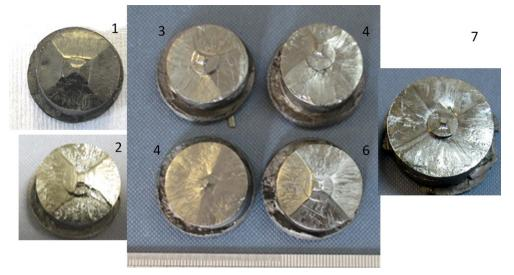
Fig. 2. Fully grown, recycled Y-Ba-Cu-O samples.
