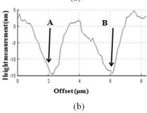
Fig. 4 (a)3D - AFM image of channel crack path of (50 nm) IGZO/PEN sample, white arrows show straining direction; (b) Cross section view of the channelling crack of (50nm) IGZO/PEN.
