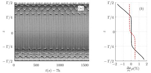
FIGURE 10. Instability of the stratified layers in the HS case with  $(\alpha, Ri_l) = (0.5, 2)$ . (a) Spatio-temporal diagram of shadowgraph. (b) Density profiles (deviation with respect to the mean  $\rho_0$ , nondimensionalised by  $\rho_0$ ), at mid-gap  $r = 1/2(r_i^* + r_o^*)$  from conductivity measurements, at t = 0 (solid line) and t = 40 h (dashed line): the SRI destroys the initial density profile in a few diffusion time units.
