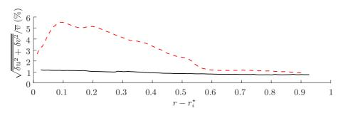
FIGURE 6. PIV measurements of horizontal turbulence intensity at the equator, in the absence of stratification. Comparison between the HS case (dashed red line) and the LS case (solid black line).
