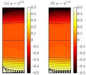
FIGURE 9. Base flow density field  $\rho_B$  in (a) HS case (unstable) and (b) LS case (stable);  $(\alpha, Ri_l) = (0.5, 2)$ . Dotted lines mark the limits of the stratified layers. Density step between solid lines: 0.05; between dashed lines:  $5 \times 10^{-3}$ .
