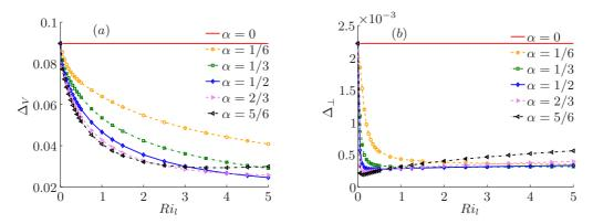
FIGURE 8. (a) Relative azimuthal deviation  $\Delta_V$  and (b) relative meridional deviation  $\Delta_{\perp}$  as functions of  $R_{l_l}$ , for various values of  $\alpha$ , in the LS case.
