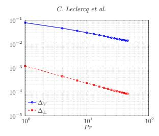
FIGURE 12. Effect of the Prandtl number on the deviations  $\Delta_V$  and  $\Delta_{\perp}$  for the HS case  $\mu = \eta^{3/2}, \ \alpha = 0.5$  and  $Ri_l = 2$ .
