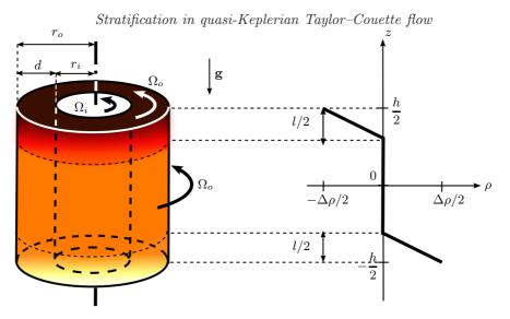
FIGURE 1. Partially stratified Taylor–Couette setup: the flow is linearly stratified in the axial direction z near the end-plates (colour scheme is indicative of temperature). In this paper, the end-plates are attached to the outer cylinder. Rather than the total density,  $\rho$  denotes the deviation with respect to a reference value  $\rho_0$ .
