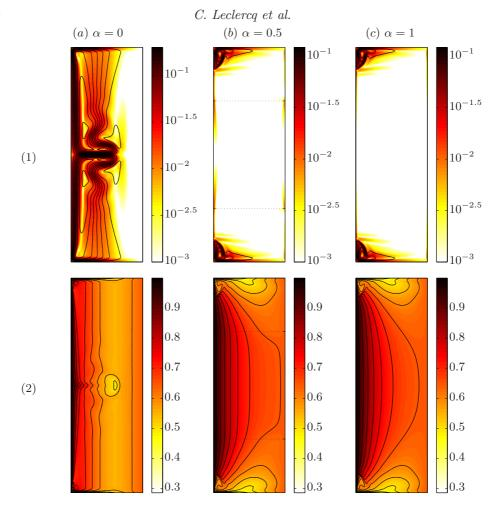
FIGURE 3. Base flow for the HS case  $\mu = \eta^{3/2}$  (1) Meridional flow  $\mathbf{U}_{\perp} = (U, W)$ : streamlines  $(\Delta \psi = 10^{-3})$  and colourmap of the norm  $\|\mathbf{U}_{\perp}\|$ . (2) Azimuthal velocity V: colourmap and contours of V ( $\Delta V = 0.05$ ). Dotted lines in (b) indicate the limit of the stratified layers. In this figure and hereafter, the left (resp. right) boundary corresponds to the inner (resp. outer) cylinder.
