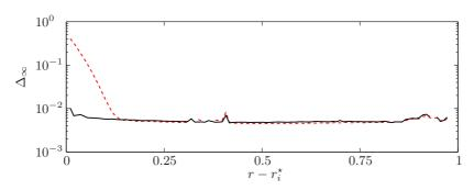
FIGURE 14. Deviation  $\Delta_{\infty}$  from the unperturbed state at the equator when searching for subcritical transition to turbulence. The dashed curve shows a measure of  $\Delta_{\infty}$  right after applying the pertubation and the solid line corresponds to the deviation 30 min later. For this forcing at  $Re = O(10^4)$ , turbulence is not triggered in the unstratified zone as is evident from the low values of  $\Delta_{\infty} \approx 1\%$  rapidly reached.
