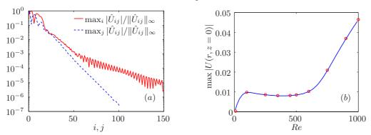
FIGURE 2. (a) Convergence of spectral coefficients  $U_{ij}$  of the radial velocity component, for  $\mu = \eta^{1/2}$ ,  $\alpha = 0.5$  and  $Ri_l = 2$ . (b) Maximum radial velocity at the equator for  $\eta = 0.5$ ,  $\Gamma = 6$ ,  $\mu = 1$ , fixed end-plates and no stratification. Solid line: data digitized from Avila *et al.* (2008), dots: present code.
