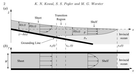
FIGURE 1. Schematic illustrating (a) the side profile and (b) the plan view of a viscous fluid layer confined between two parallel side walls and intruding into an inviscid ocean.
