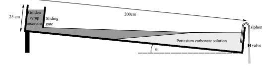
FIGURE 5. Schematic of our experimental setup. Golden syrup is kept at a constant head in the reservoir and flows under the sliding gate to form a viscous gravity current. The current flows down the sloping base of the tank into a denser solution of potassium carbonate. The level of the solution is kept constant by a siphon.
