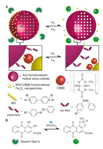
Fig. 1 Schematic illustration of a light-controlled nanocontainer composed of a hollow silica colloid as the core and Fe<sub>3</sub>O<sub>4</sub> nanoparticles as coronas. (A) HMRCs obtained through the formation of (MV/trans-Azo)⊂CB[8] heteroternary complexes and the light-driven reversible disassembly of the HMRCs. (B) A model reaction between boronic acid and Alizarin Red S.
