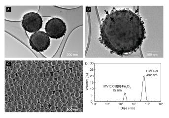
**Fig. 3** Formation of the HMRCs through CB[8]-directed self-assembly. (A) TEM image of the HMRCs. (B) A zoom in image of an HMRC with arrows indicating the shell of the hollow silica colloid. (C) SEM image of the HMRCs cast onto a glass slide. (D) DLS result of the HMRCs formed by the addition of 8 mL Azo-silica colloidal dispersion into 1 mL MV-Fe $_3$ O $_4$  nanoparticles/CB[8].
