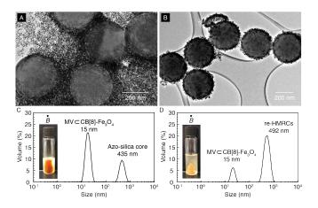
**Fig. 4** The light-driven reversible assembly of the HMRCs. TEM images of (A) the disassembled HMRCs and (B) reassembled HMRCs. DLS results of (C) the disassembled HMRCs and (D) reassembled HMRCs. The inset photos show the magnetic response of the suspensions of disassembled HMRCs and reassembled HMRCs.
