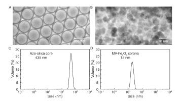
**Fig. 2** Preparation of Azo functionalized hollow mesoporous silica colloids and MV functionalized  ${\sf Fe_3O_4}$  nanoparticles. TEM images of (A) hollow mesoporous Azo-silica colloids and (B) MV-Fe<sub>3</sub>O<sub>4</sub> nanoparticles. DLS results of (C) hollow mesoporous Azo-silica colloids and (D) MV-Fe<sub>3</sub>O<sub>4</sub> nanoparticles.
