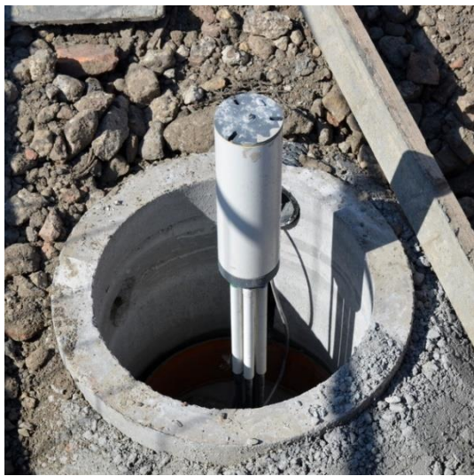
Figure 4 – a) Schematic view of rod extensometer borehole, b) Photograph of reference head, c) Schematic view of magnet extensometer borehole, d) Photograph of spider magnet anchor ( http://nvm.ie/products/geo-xm-magnetic-settlement-systems/ Accessed 04 April 2016)
