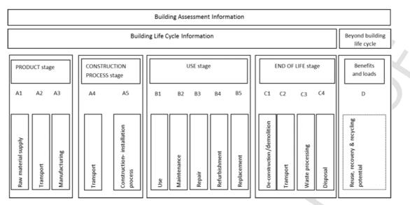
Fig. 1. Life cycle stages of a building (BS EN 15978:2011).
