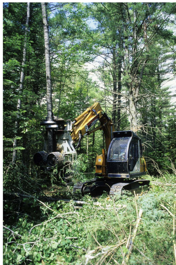
Fig. 10. Typical mechanical timber harvester head displaying gripper and debarking rollers. Wisconsin Department of Natural Resources.
