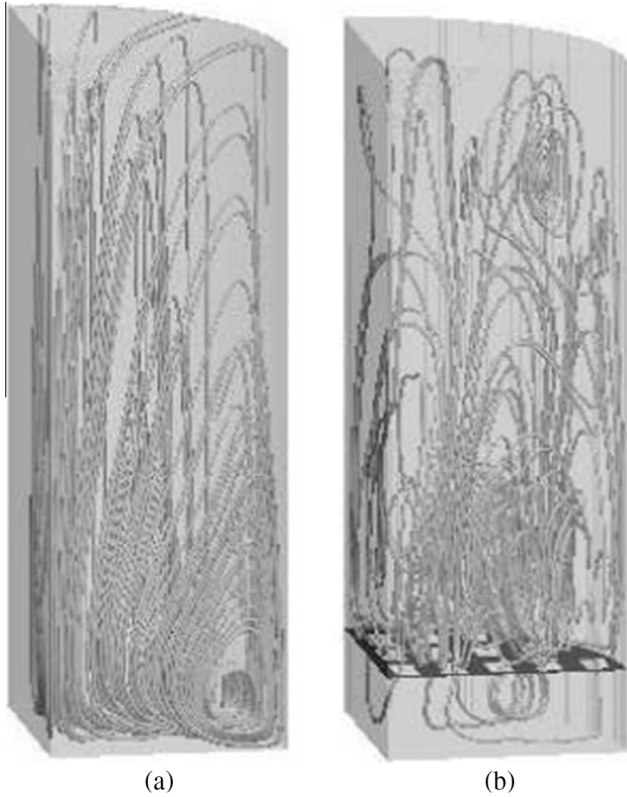
Fig. 12. Streamlines at TDC without and with grid.
